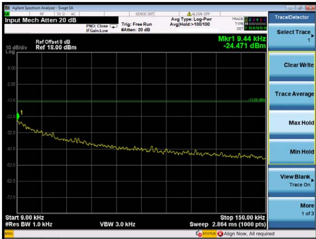
(Plot 4.6.2 B1: Channel 4183: 836.60 MHz @ WCDMA Band V)
