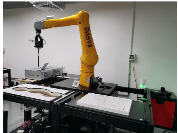
Picture D.6 Specific Absorption Rate Test Layout
