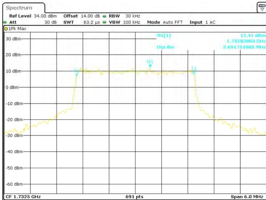
**16-QAM (3.0 MHz) - 26 dB Bandwidth, Middle channel**
