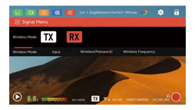
Select the Signal Menu – Wireless Mode interface, switch TX or RX mode according to your needs, and the current status will be displayed in the status bar at the bottom.
