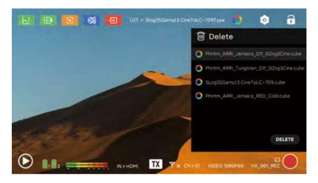
You can only delete the LUT in the monitor, the LUT on the shortcut key cannot be deleted. You need to restore the factory setting, or select a new LUT to overwrite. The LUT in the TF card also cannot be deleted, the only option is to format the memory card.
