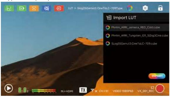
Select the LUT in the TF card and click import, it will be prompted that the current LUT shortcut key can be overwritten during import. If the LUT shortcut key is not currently selected, it will be loaded into the monitor (the monitor can save up to 50 LUTs).
