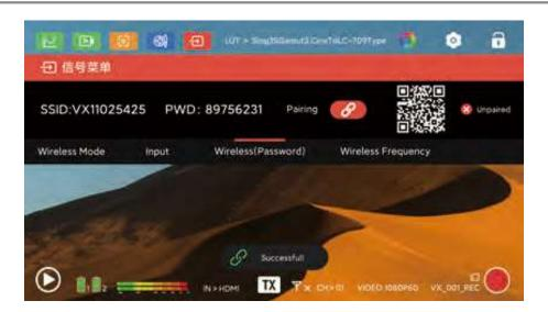
Enter the Settings – System Information interface, select Wireless Information. Then open the mobile App to Connect Device, select Scan Code to connect, and scan the QR code on the monitor to connect.
