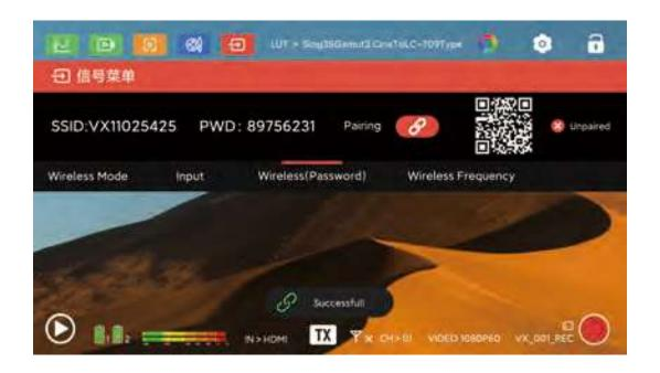
Enter the Signal Menu – Wireless Information interface, click the pairing button both on TX & RX simultaneously to pair. The pairing method is the same in TX or RX mode.
