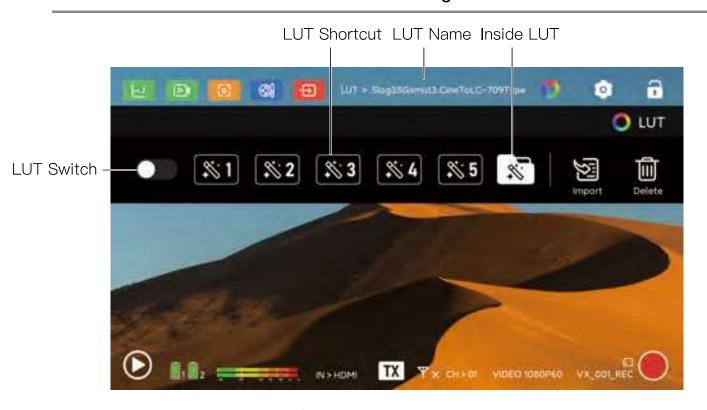
Put the LUT file into the TF card (LUT format is \*.cube, support 17x17x17 and 32x32x32), select the import button
