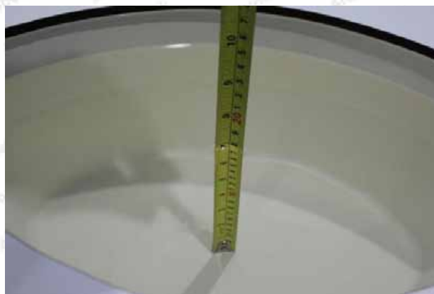
Liquid depth in the body phantom (5GHz)
