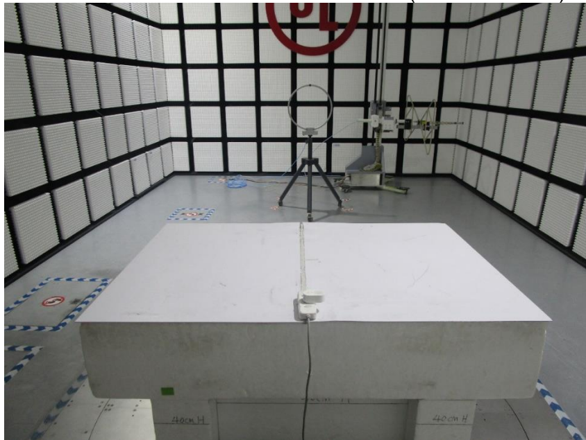
RADIATED RF MEASUREMENT SETUP (BELOW 30MHz)
