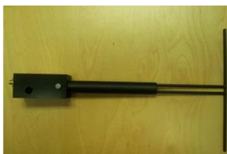
Figure 1 – MVG COMOSAR Validation Dipole
