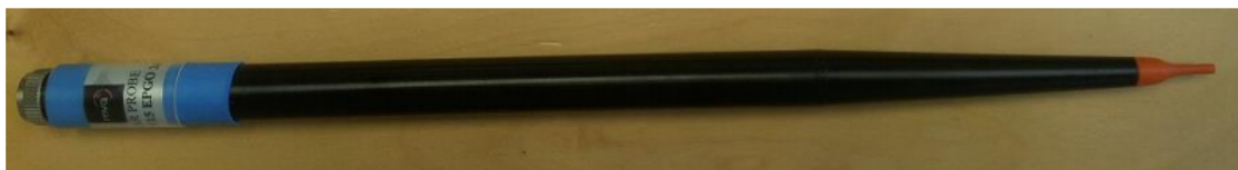
Figure 1 – MVG COMOSAR Dosimetric E field Dipole
