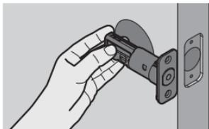
Hold the latch in front of the bore hole, with the latch face flush against the door edge. Is the slotted hole centered in the door hole?
