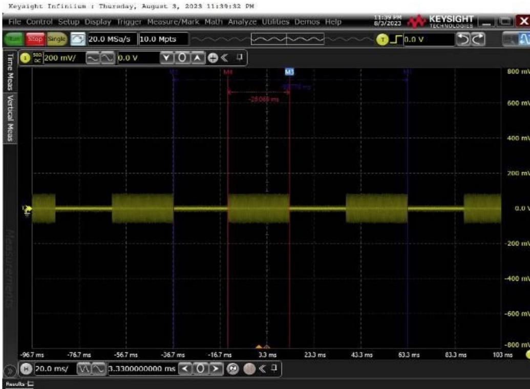
Blue marks showing a 100ms duty-cycle, during that we are executing two transmits.
