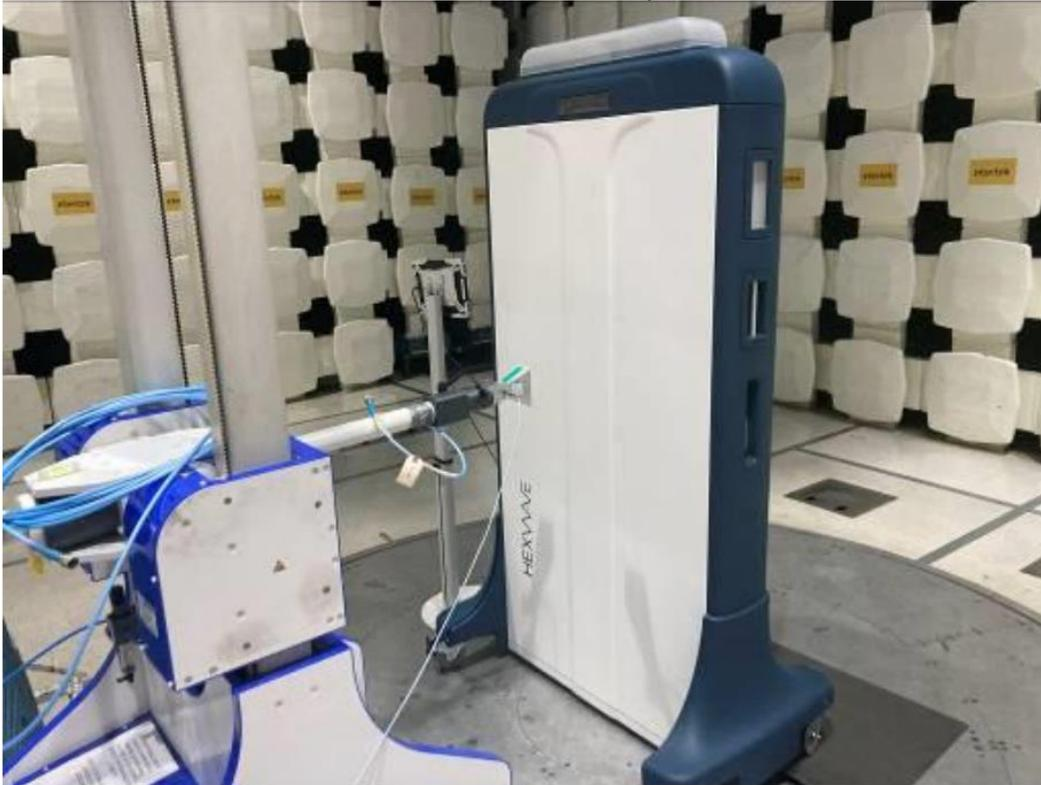
40-60 GHz Test Setup
