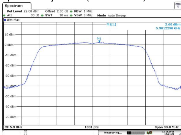
Power Spectral Density Data Plot (CH Mid 5300 MHz)
