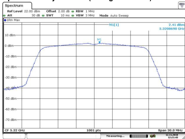
Power Spectral Density Data Plot (CH High 5320 MHz)
