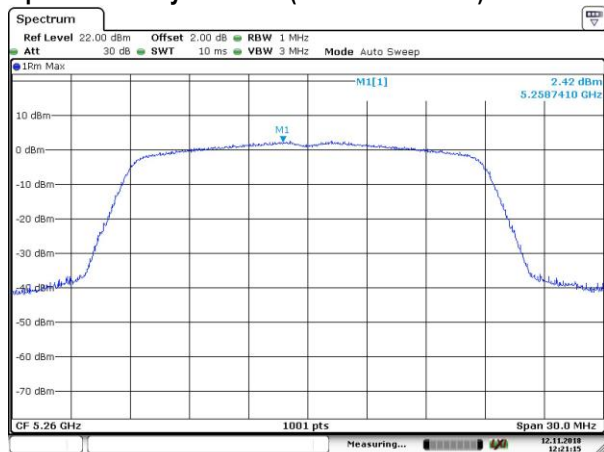
802.11n HT20, 5250~5350 MHz Power Spectral Density Data Plot (CH Low 5260MHz)
