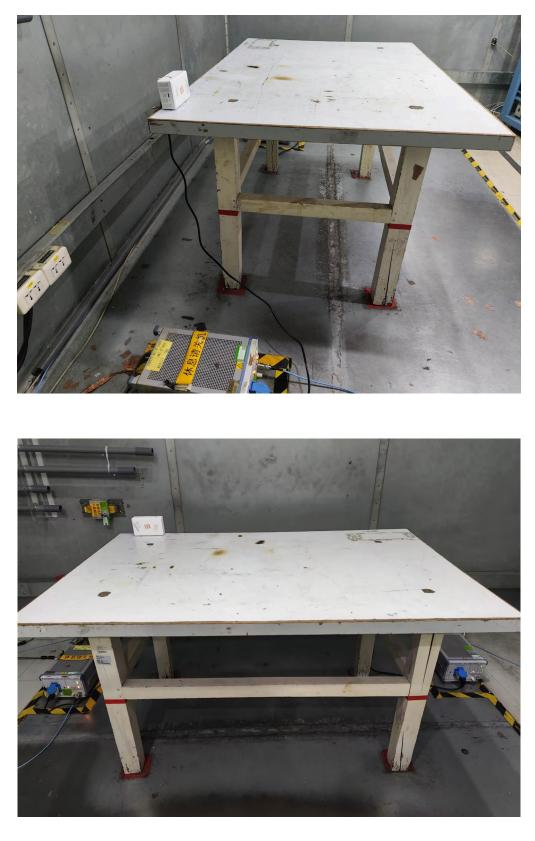
AC Power Line Conducted Emissions Test Photos
