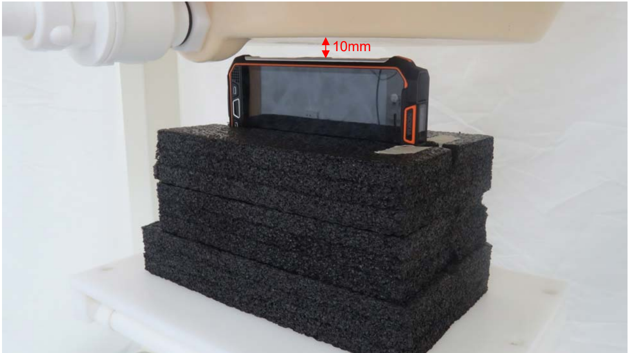
Picture 9: Left Edge, the distance from handset to the bottom of the Phantom is 10mm
