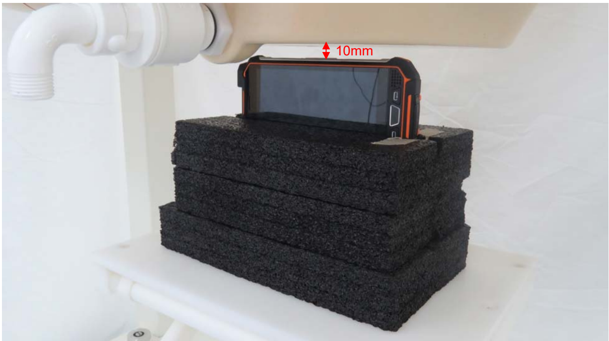
Picture 10: Right Edge, the distance from handset to the bottom of the Phantom is 10mm
