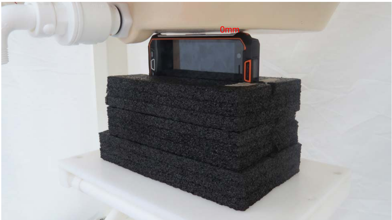
Picture 14: Left Edge, the distance from handset to the bottom of the Phantom is 0mm
