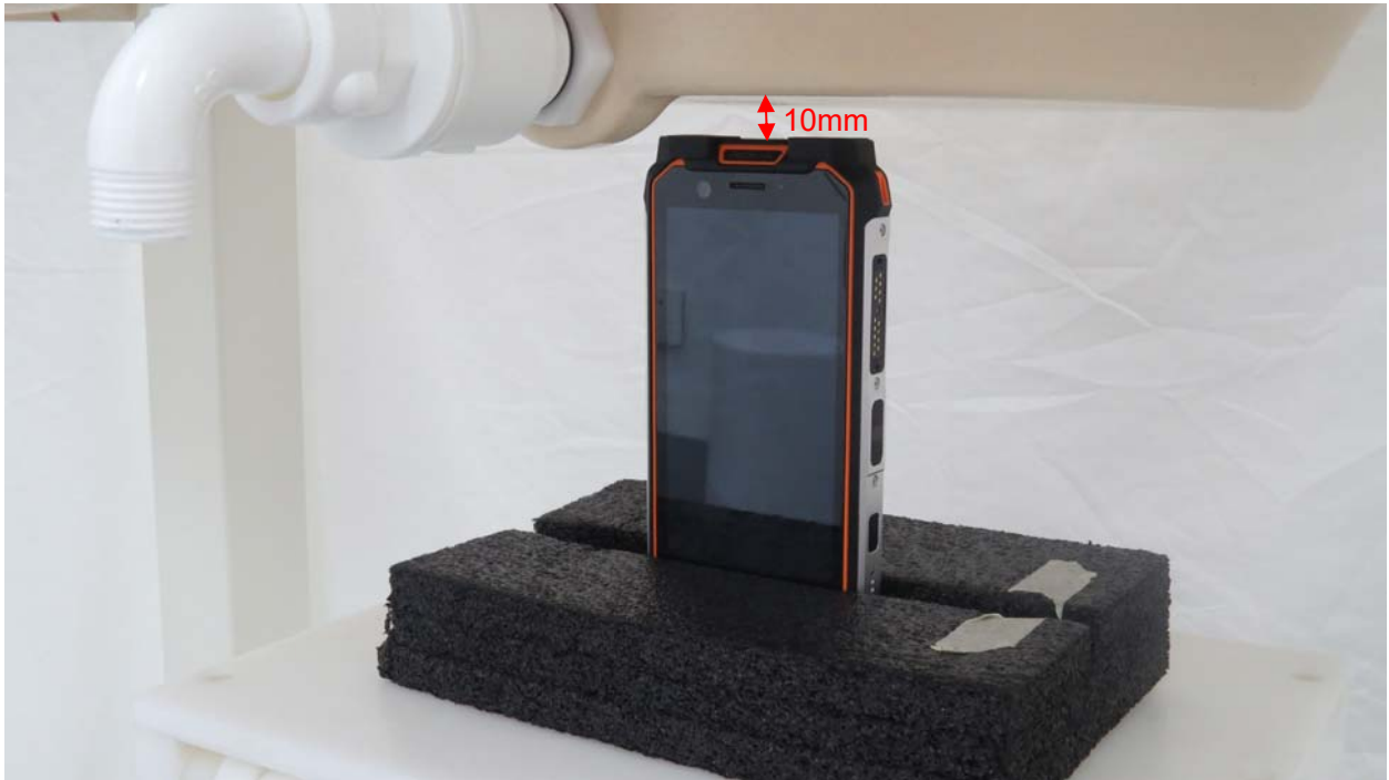
Picture 11: Top Edge, the distance from handset to the bottom of the Phantom is 10mm
