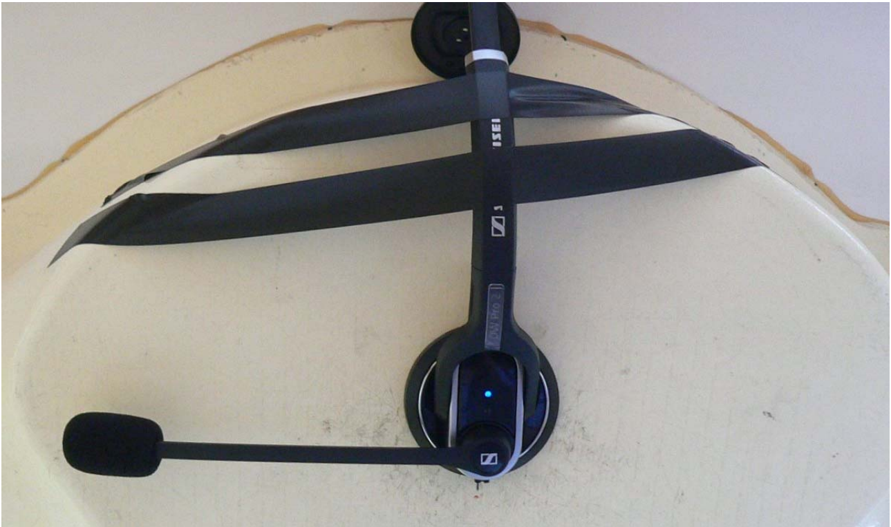
Fig. 13: Test position 1 for the DW 30 HS from Sennheiser Communications, bottom view.
