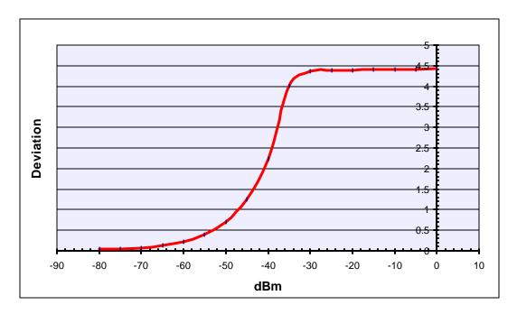
Modulation Limiting for 1000Hz
