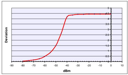
Modulation Limiting for 2500Hz
