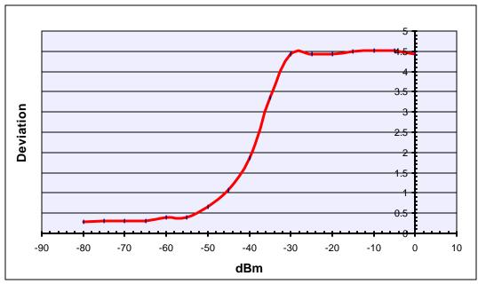
Modulation Limiting for 300Hz
