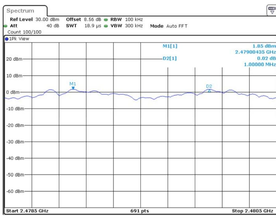
**EDR (8DPSK): Low Channel**
