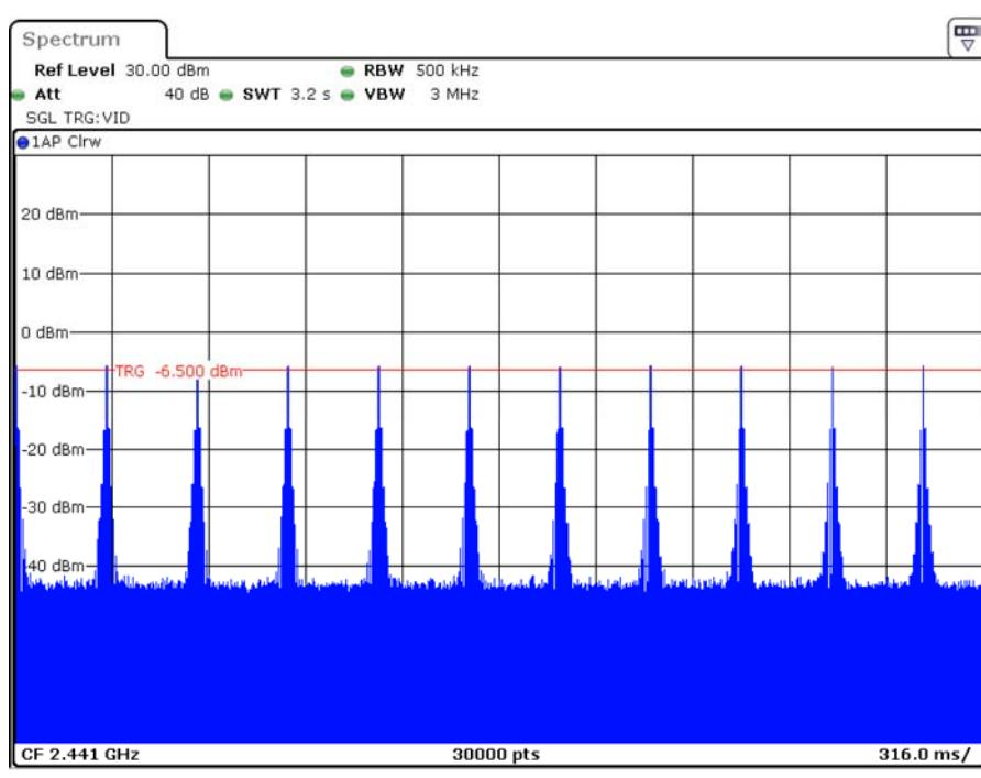
**EDR (8DPSK):****Pulse Time, 3DH1, 2441 MHz**
