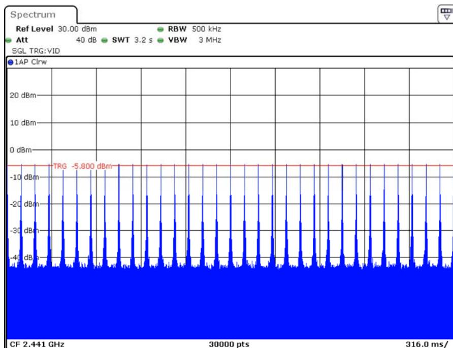
**Pulse Time, 3DH3, 2441MHz**
