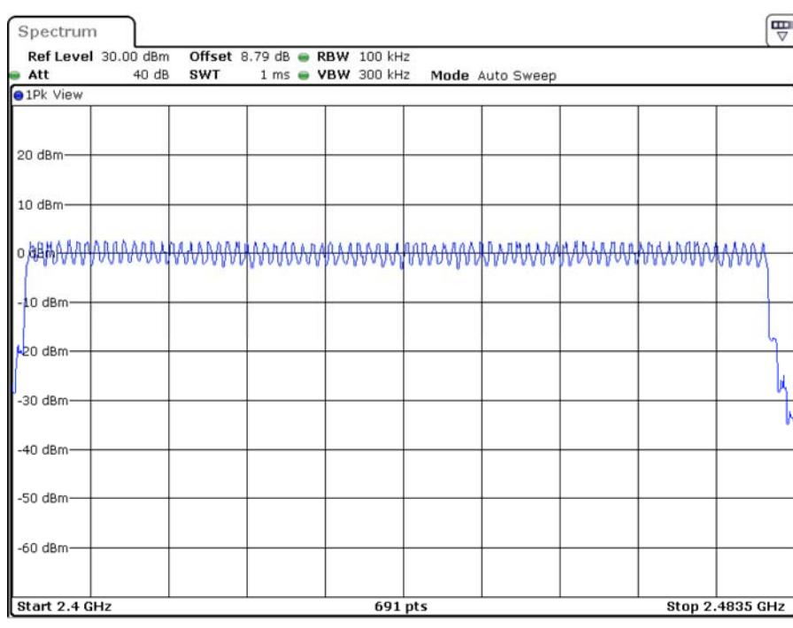
**EDR (8DPSK): Number of Hopping Channels**
