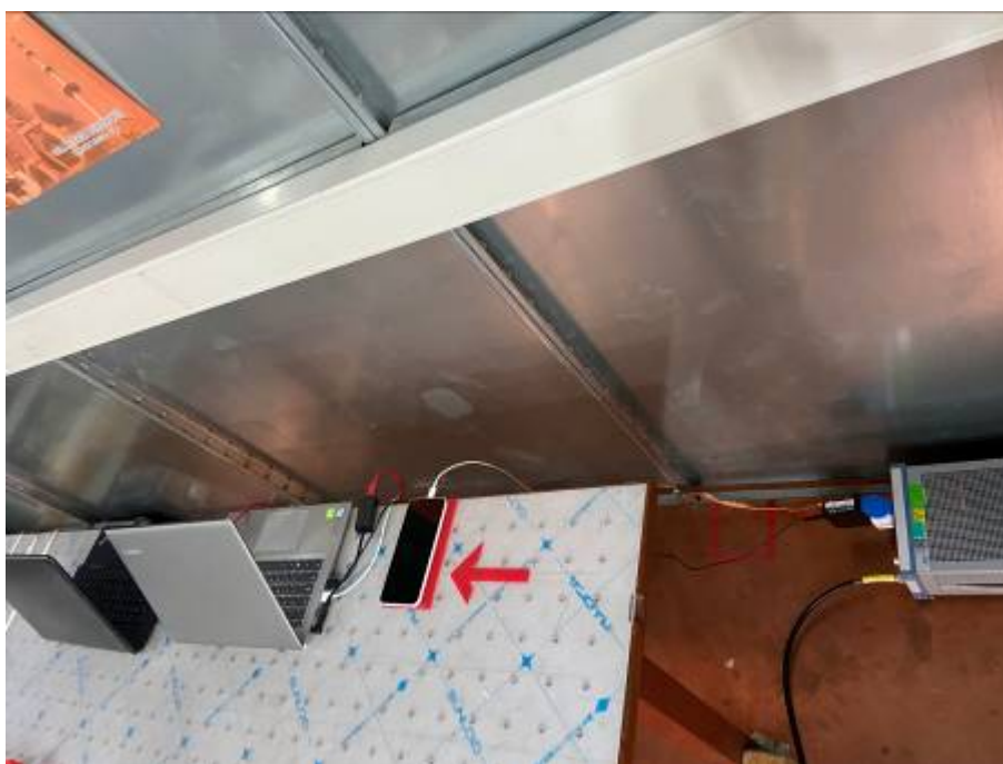
Conducted Emissions Test Setup (with laptop)
