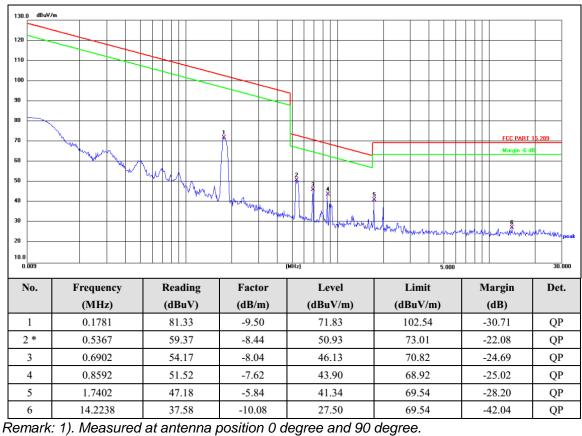
2). Corrected Reading: Antenna Factor + Cable Loss + Read Level - Preamp Factor = Level.
