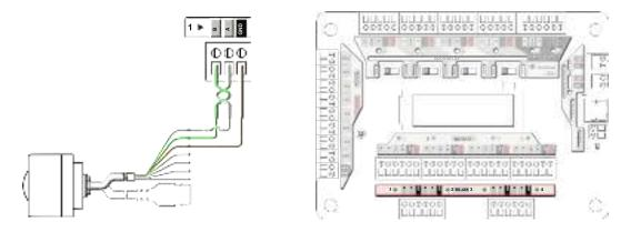
Power to the reader can be supplied using POE or a 12-28VDC external power source. DR40 has a maximum current rating of 791 mA at 12VDC, so should not be power directly by the DC20. Always check the power requirements of the door controller prior to installation. If PoE is not used, an Ethernet or Wi-Fi connection is required. Refer to Recommended Wire Type and Size table above for more wiring detail.
