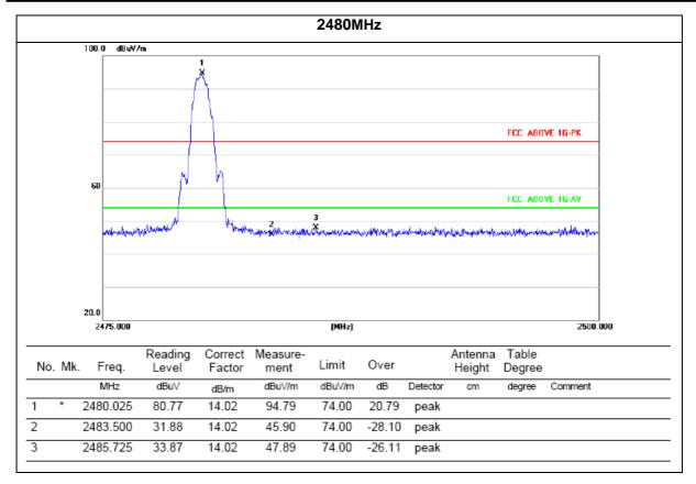
If the PK measured levels comply with average limit, then the average level were deemed to comply with average limit.
