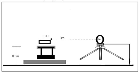
(B) Radiated Emission Test-Up Frequency 30MHz~1GHz
