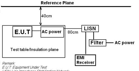
LISN: Line Impedence Stabilization Network Test table height=0.8m
