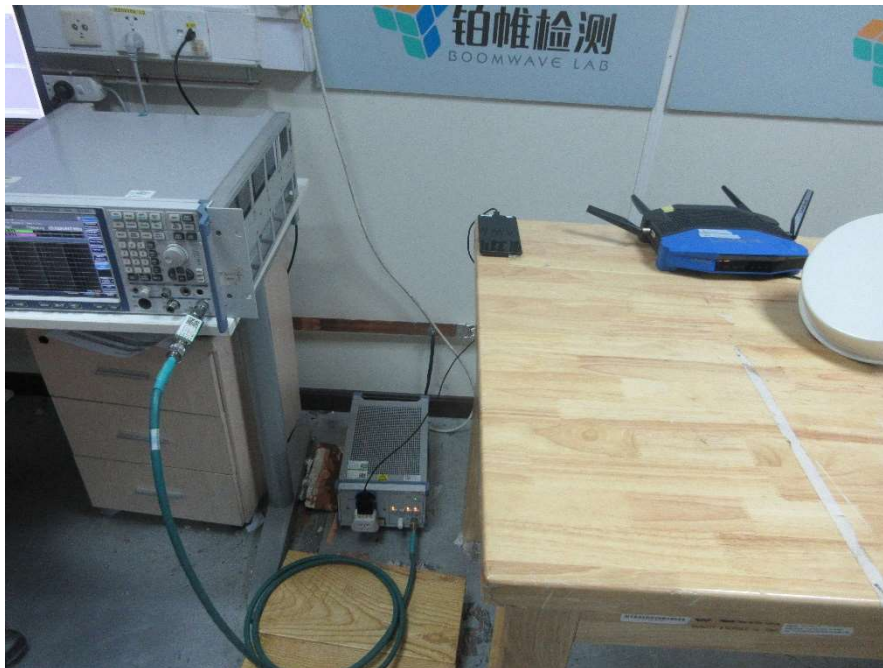
Conducted Emission 150kHz-30MHz (Front view) – Mode 2
