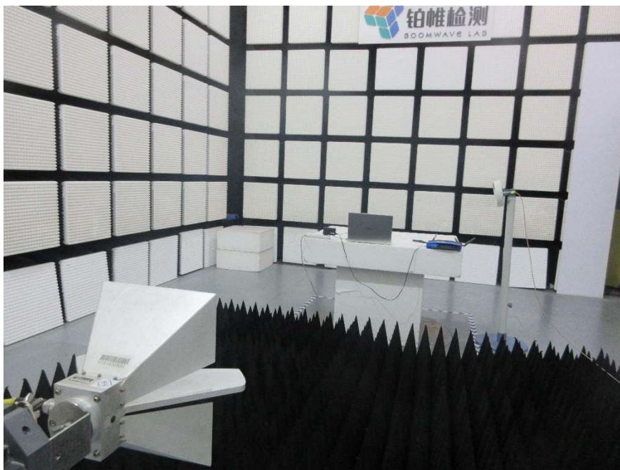
Radiated Emission 1GHz-18GHz (Rear view) – Mode 5
