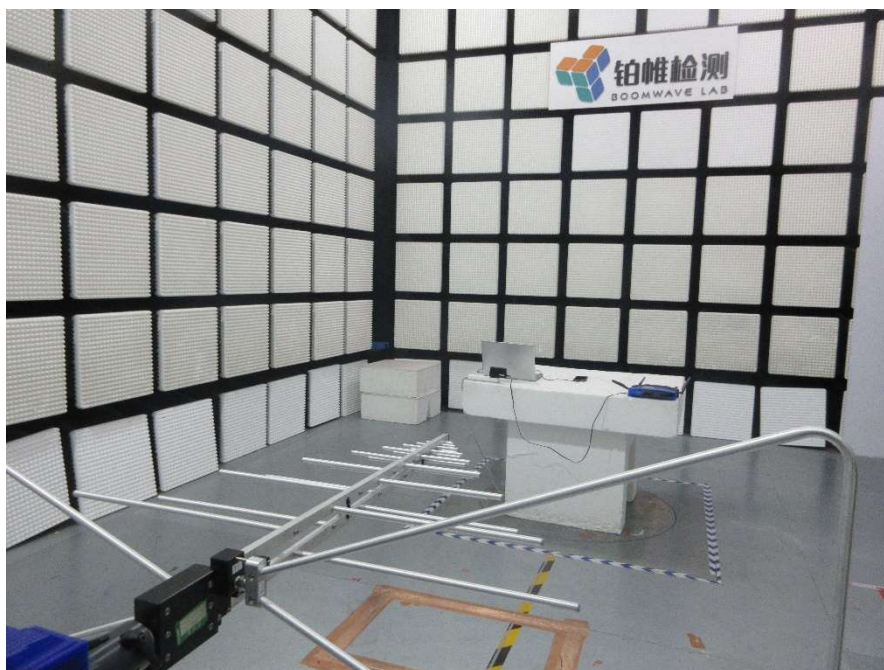
Radiated Emission 30MHz-1GHz (Rear view) – Mode 5
