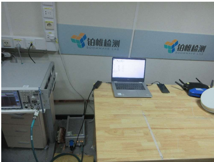
Conducted Emission 150kHz-30MHz (Front view) – Mode 5
