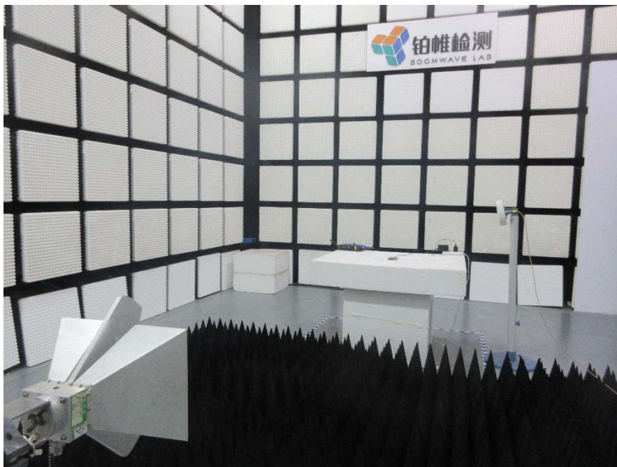
Radiated Emission 1GHz-18GHz (Front view) – Mode 2
