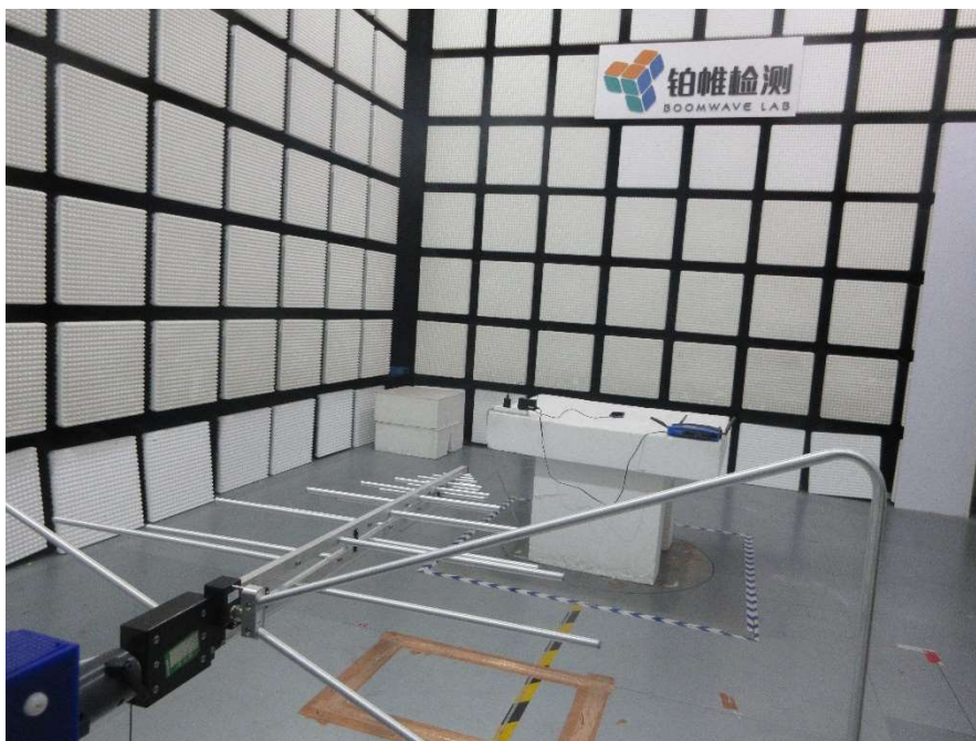
Radiated Emission 30MHz-1GHz (Rear view) – Mode 2
