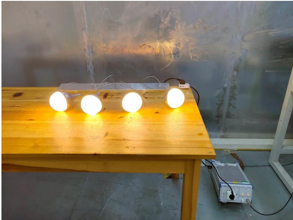
Photo of Power Line Conducted Measurement
