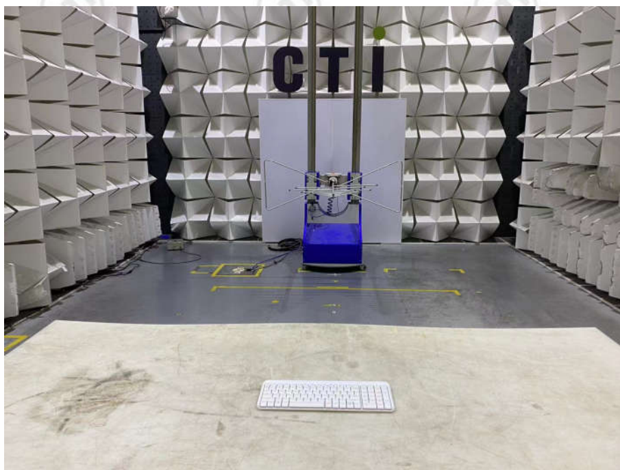
Radiated spurious emission Test Setup-1(Below 1GHz)
