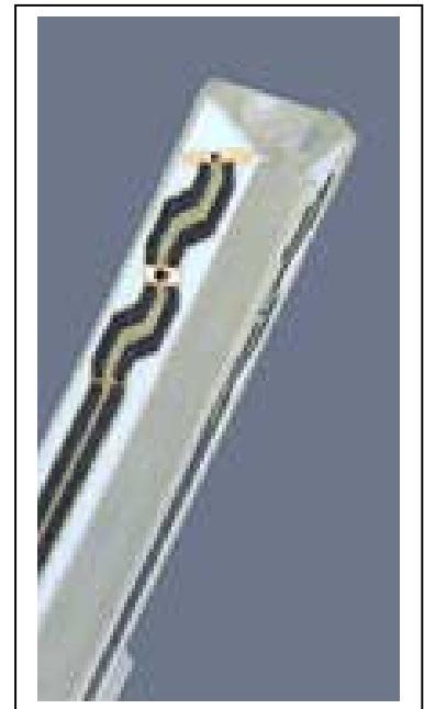
Inside view of ET3DV6 E-field Probe
