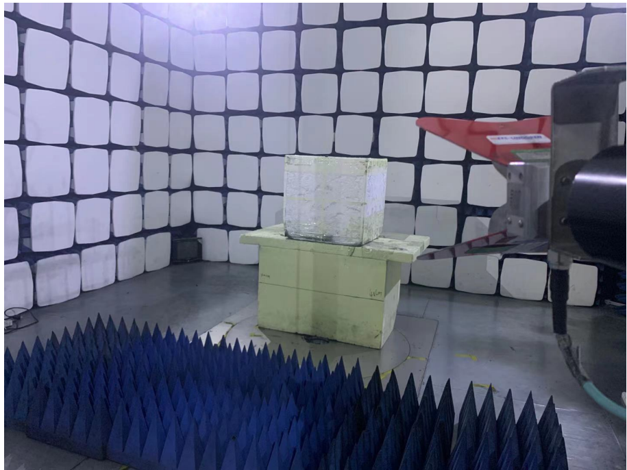
Radiation Emission Test Setup (1GHz to 18GHz)
