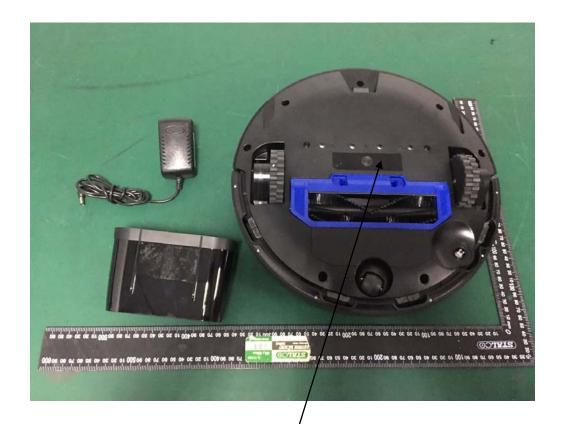
Model: LDS M6 PRO Charging Base Model:LDS M6 PRO FCC ID: 2ARZX-LDS-M6PRO Product Name: Robot Vacuum Cleaner Input: 20V === 1.2A Rated Power: 33W
