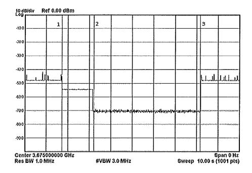
Comment: red line (1) – interferer signal is turned on, green line (2) – interferer signal is turned off, blue line (3) – the connection between the AP and SM is restored
