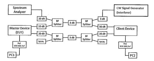
Note: for the test when a similar Canopy AP was used as an interferer, the CW Signal Generator was substituted for this AP for unlike system.
