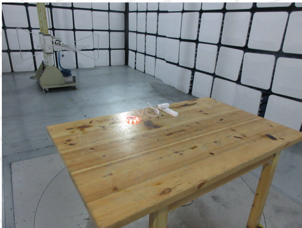
Photo of Radiation Emission Test
