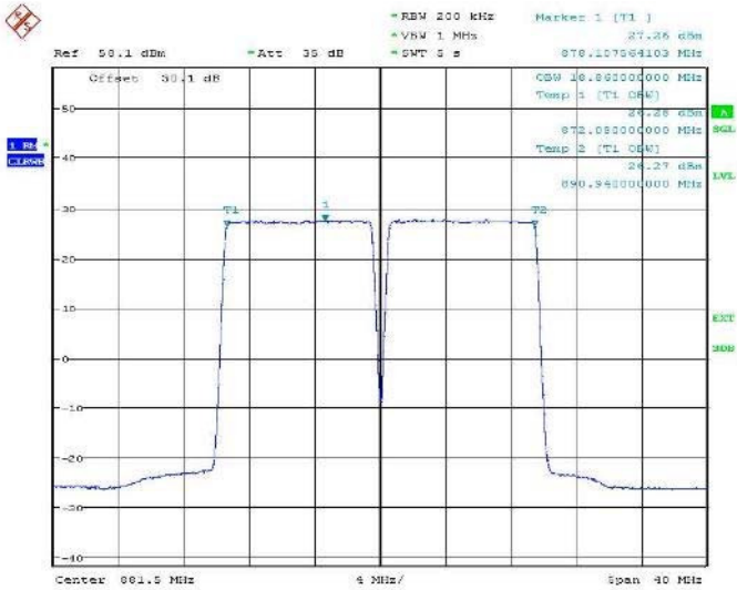
Figure 131 Occupied Bandwidth – 64QAM (876.5/886.5 MHz) (10MHz Channel BW)
