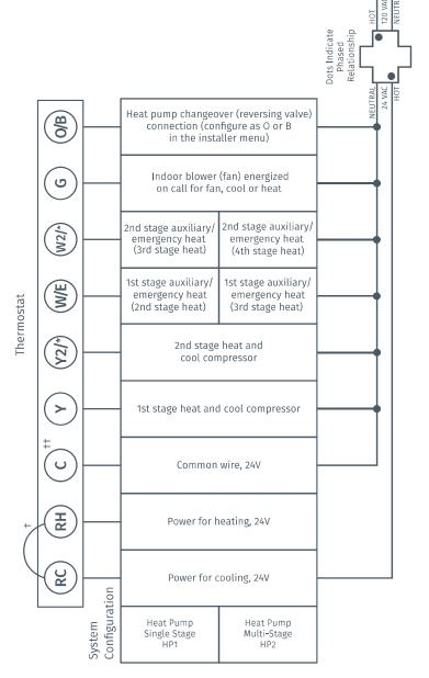
"Internal jumper between RC and RH, located on back of thermostat." Common connection required on Heat-only, Cool-only or Heat Pump systems.
