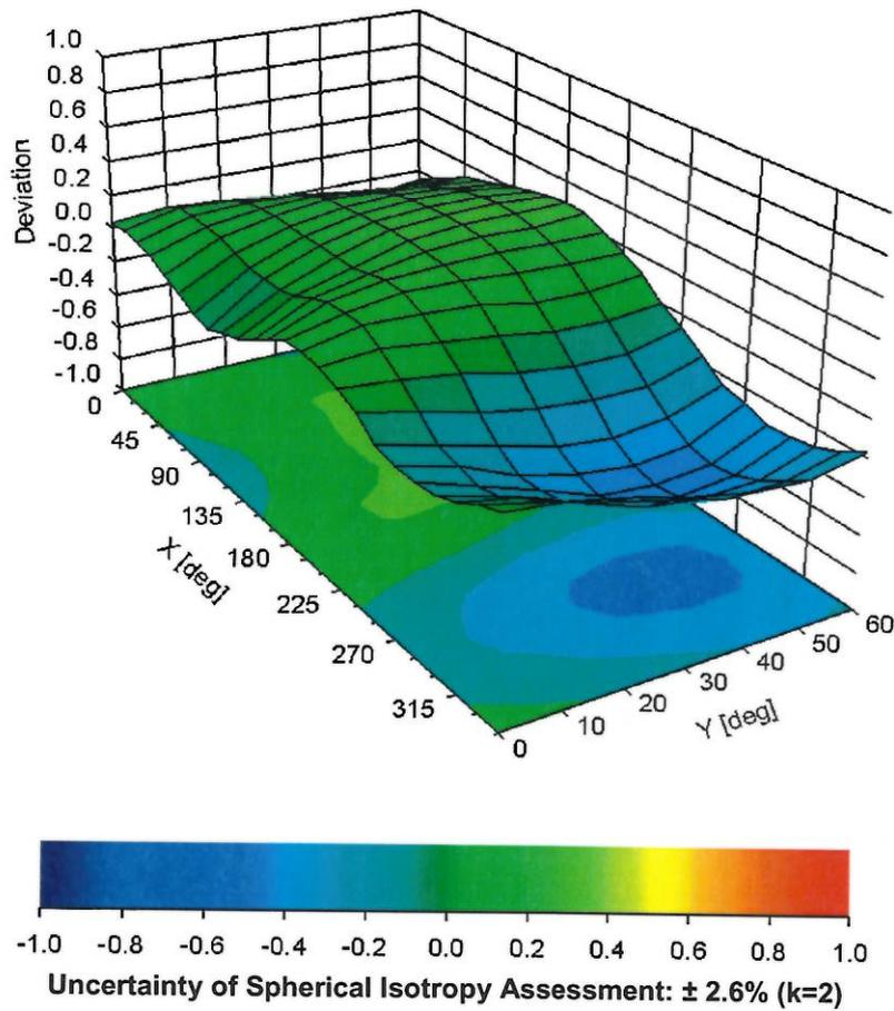
**DASY/EASY - Parameters of Probe: EX3DV4 - SN:7330****Other Probe Parameters**
