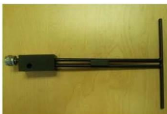
Figure 1 – MVG COMOSAR Validation Dipole
