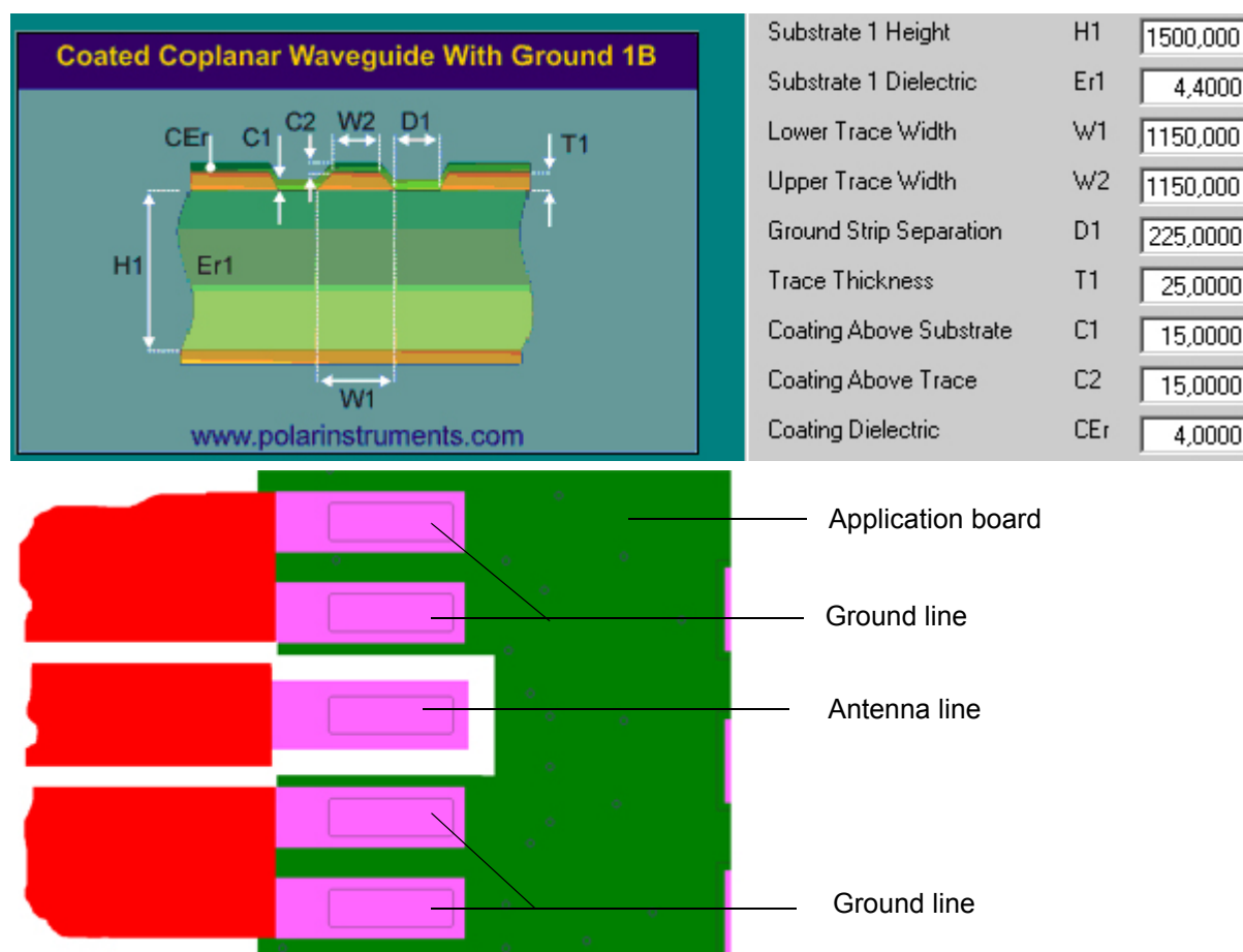
Figure 25: Micro-Stripline on 1.5mm Standard FR4 PCB - example 2
