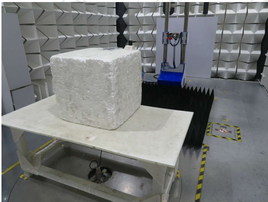
Radiated spurious emission Test Setup-3(Above 1GHz)
