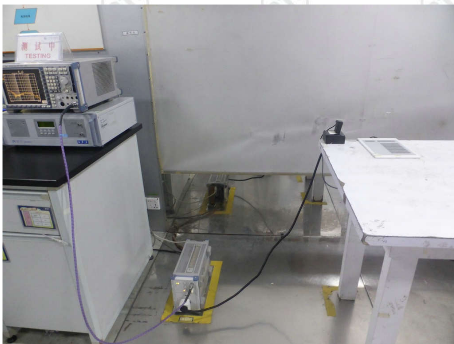
Conducted Emissions Test Setup
