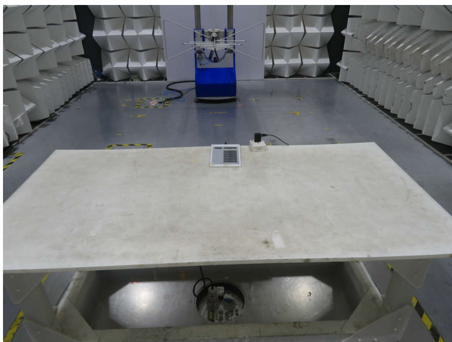
Radiated spurious emission Test Setup-2(30MHz-1GHz)
