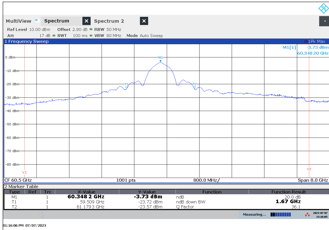
Plot 25: 20 dB-Bandwidth at T= 30 °C / V min-max
