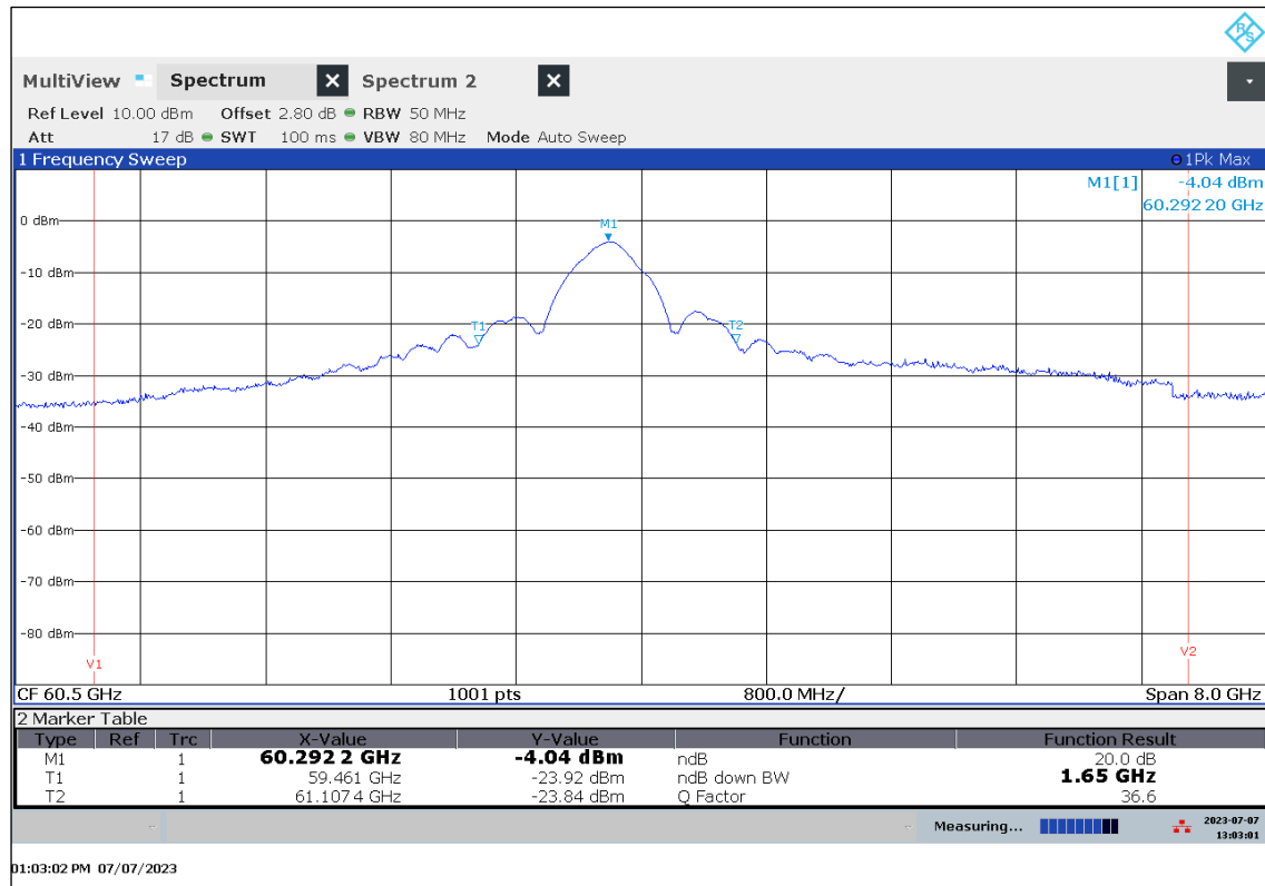
Plot 27: 20 dB-Bandwidth at T= 50 °C / V min-max
