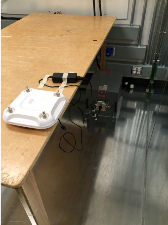
AIR-CAP3702P-B-K9 AC Conducted Emissions setup photo
