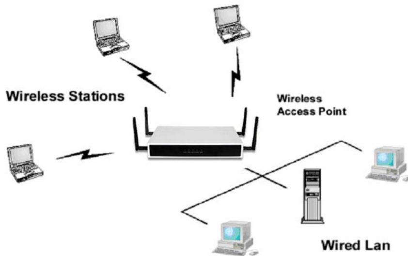
Figure 1: Wireless Access Point
