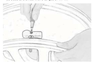
Step 3: Tighten the air nozzle fixing nut with a wrench to complete the installation. Note that the wrench uses a torque of 7 N•m.
