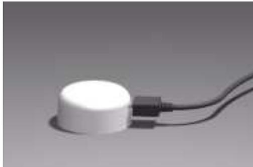
Figure 5 : AcuPebble SA100 sensor connected to micro-USB charger
