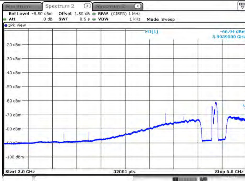
Plot on Configuration VHT80 / 5610 MHz / Average / Port 2 / 3GHz~6GHz
