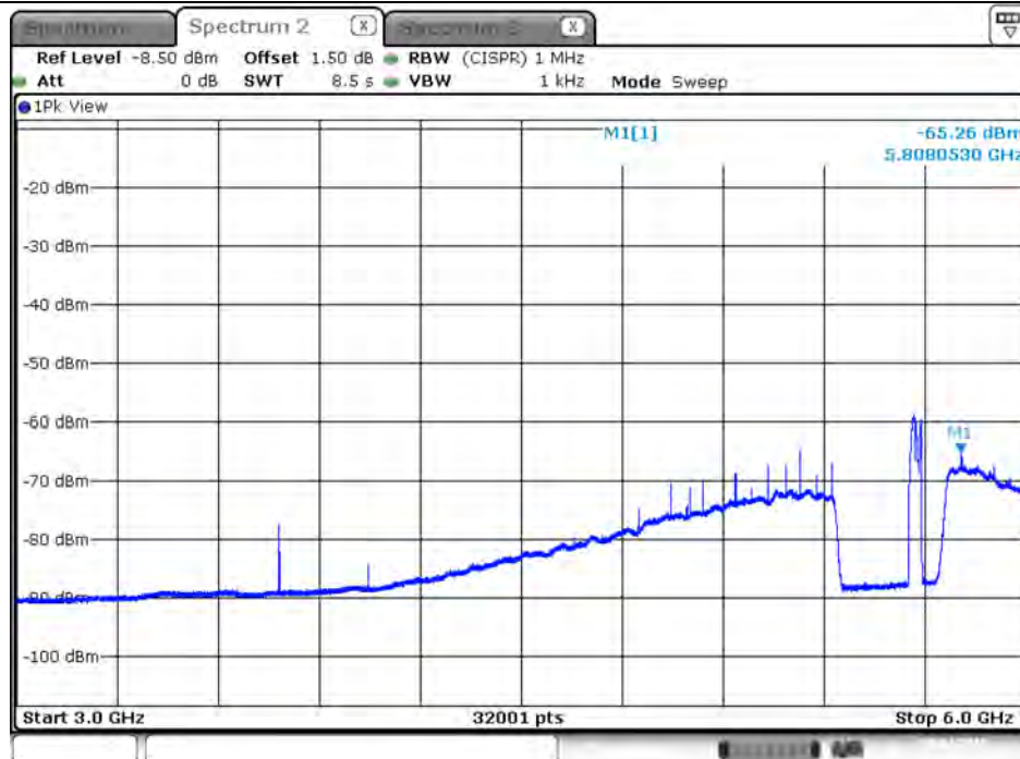
Plot on Configuration VHT40 / 5670 MHz / Average / Port 1 / 3GHz~6GHz
