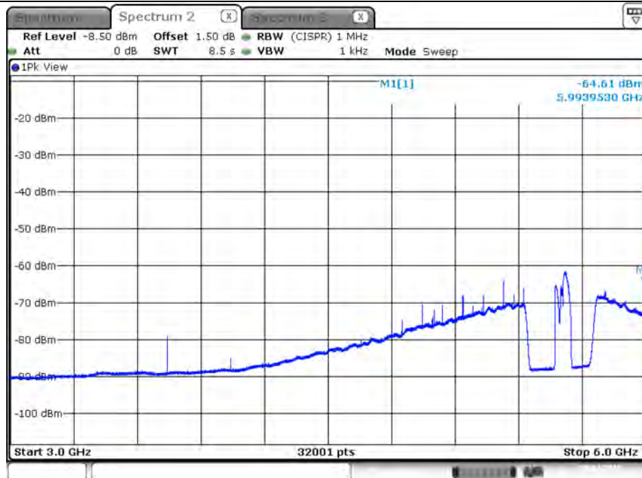
Plot on Configuration VHT80 / 5610 MHz / Average / Port 1 / 3GHz~6GHz
