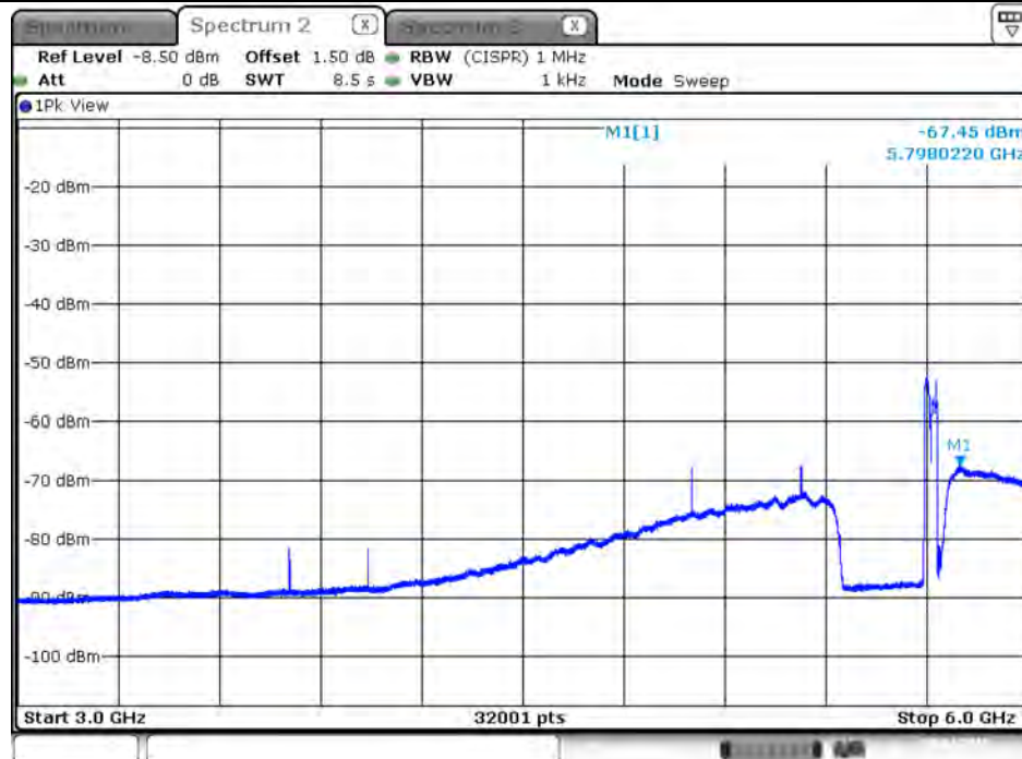
Plot on Configuration VHT40 / 5710 MHz / Average / Port 2 / 3GHz~6GHz
