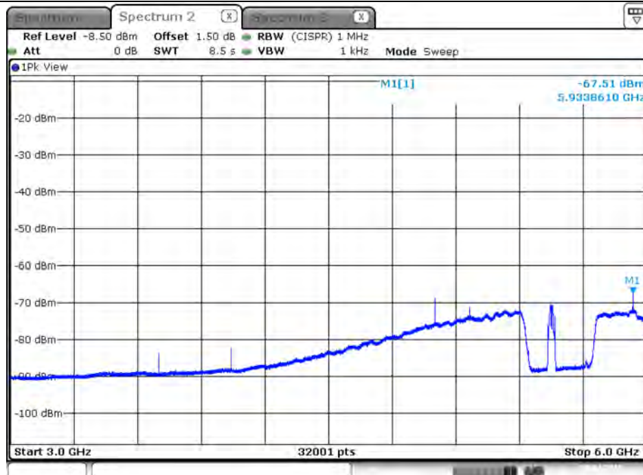
Plot on Configuration VHT40 / 5550 MHz / Average / Port 2 / 3GHz~6GHz
