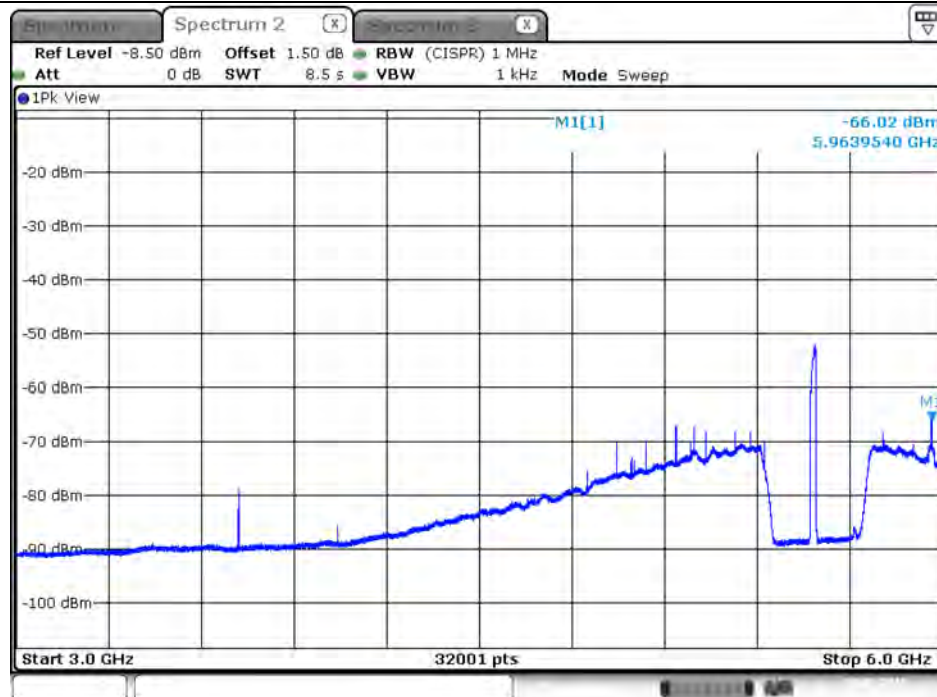
Plot on Configuration VHT20 / 5580 MHz / Average / Port 1 / 3GHz~6GHz
