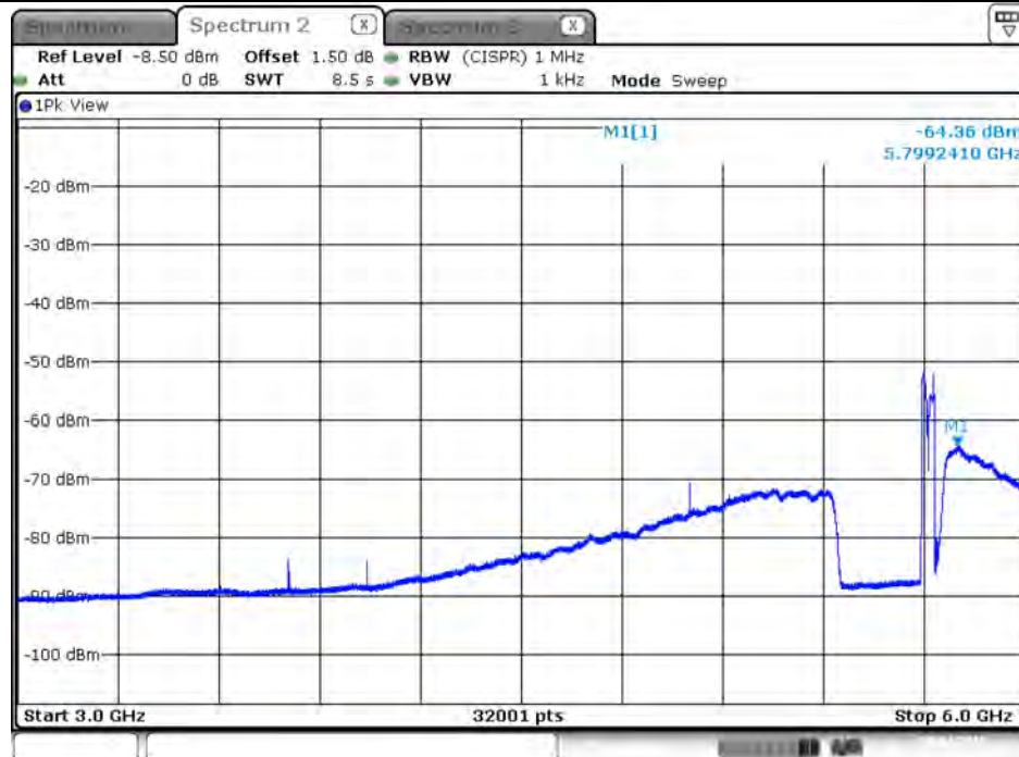
Plot on Configuration VHT40 / 5710 MHz / Average / Port 4 / 3GHz~6GHz
