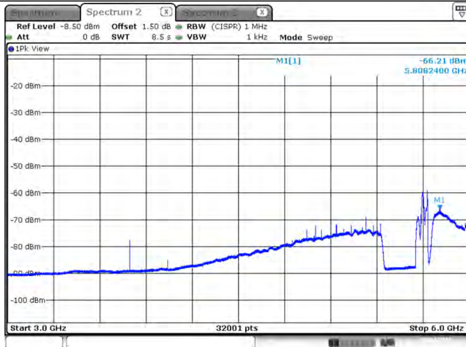
Plot on Configuration VHT80 / 5690 MHz / Average / Port 1 / 3GHz~6GHz
