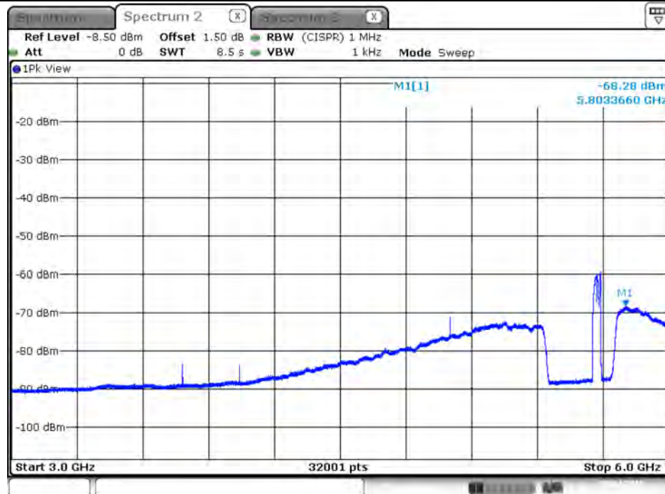
Plot on Configuration VHT40 / 5670 MHz / Average / Port 4 / 3GHz~6GHz
