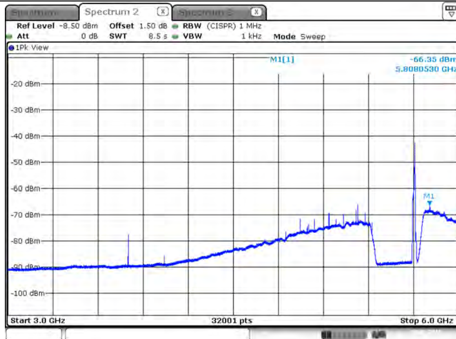
Plot on Configuration VHT20 / 5700 MHz / Average / Port 1 / 3GHz~6GHz
