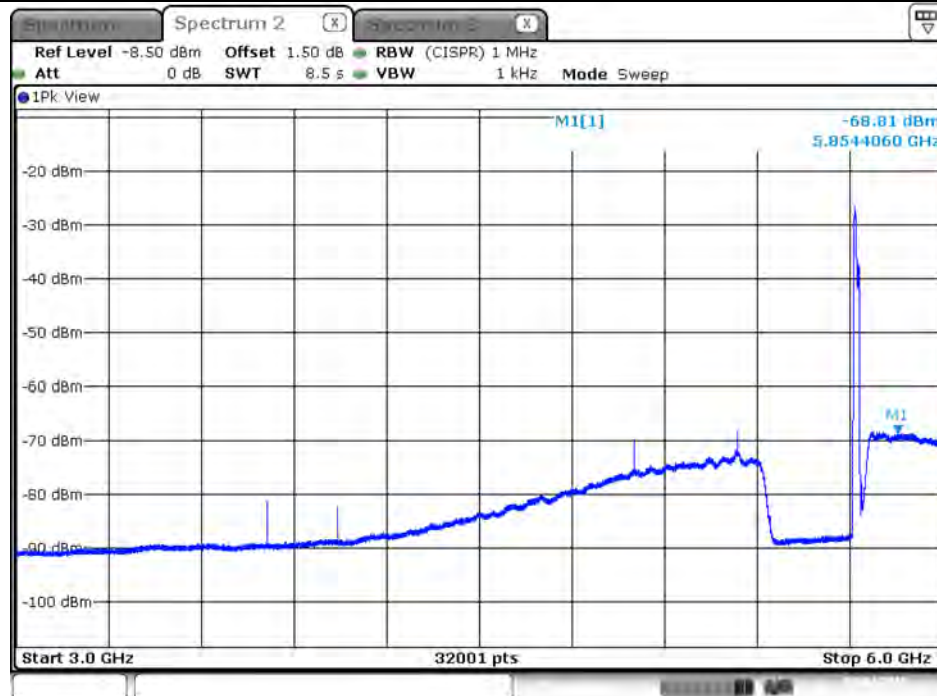
Plot on Configuration VHT20 / 5720 MHz / Average / Port 2 / 3GHz~6GHz
