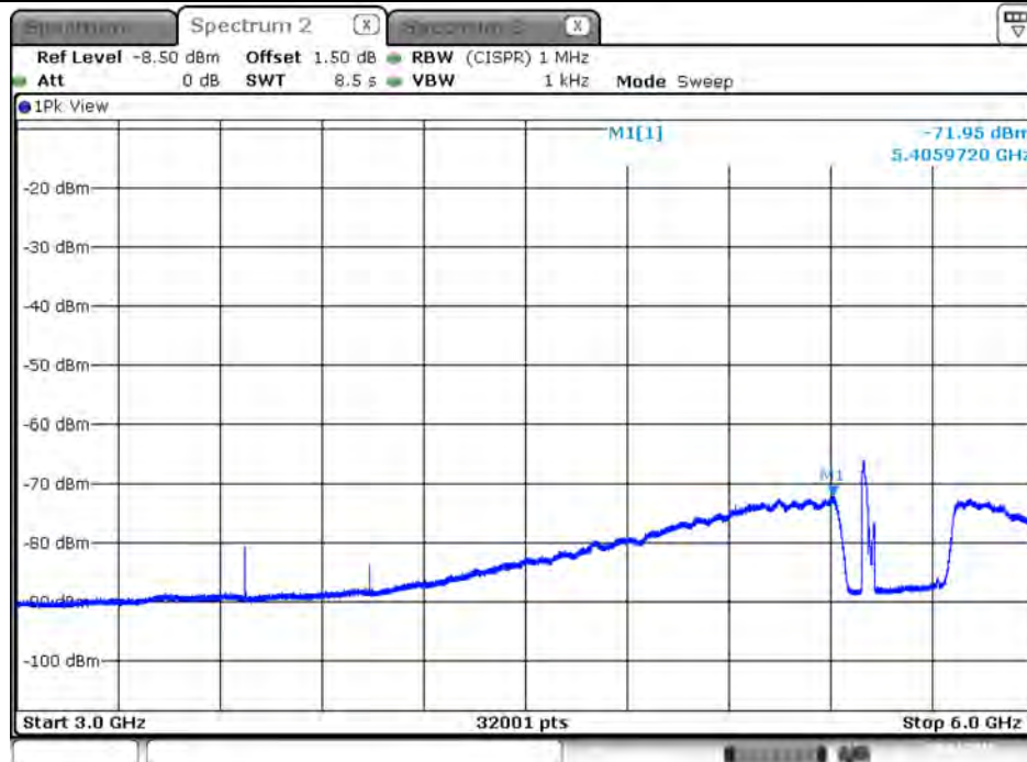
Plot on Configuration VHT40 / 5510 MHz / Average / Port 4 / 3GHz~6GHz
