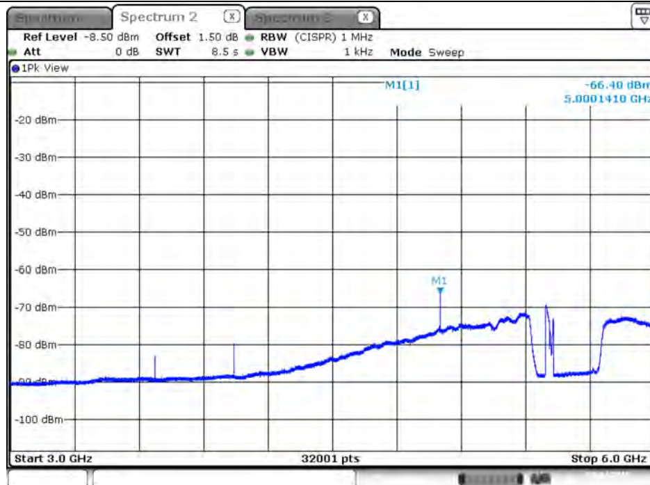
Plot on Configuration VHT40 / 5510 MHz / Average / Port 3 / 3GHz~6GHz
