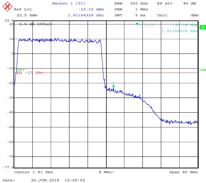
**16-QAM (20.0 MHz, FULL RB) - Left Band Edge**
