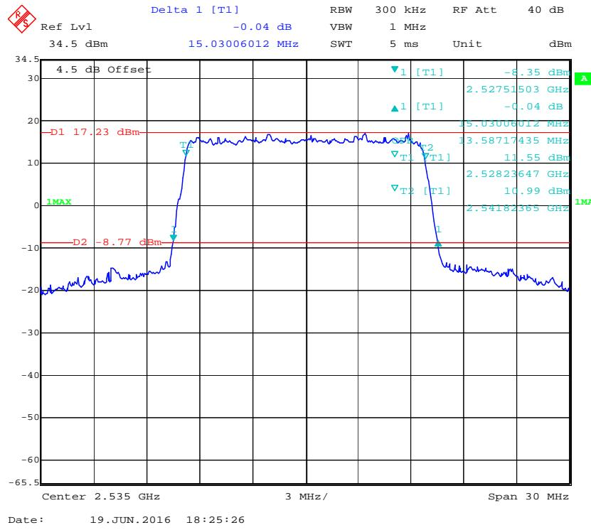
**16-QAM (15.0 MHz) - 99% Occupied Bandwidth & 26 dB Bandwidth, Middle channel**
