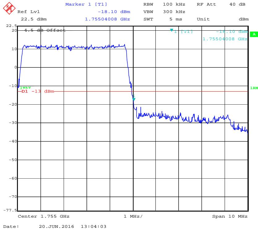
**16-QAM (5.0 MHz, FULL RB) - Left Band Edge**
