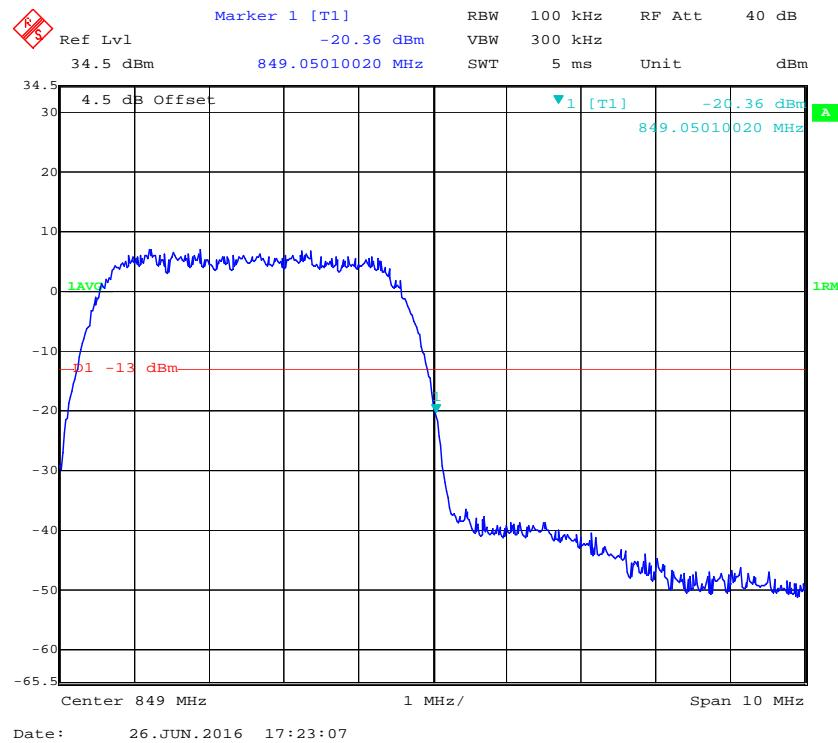
**PCS Band, Left Band Edge for GSM (GMSK) Mode**
