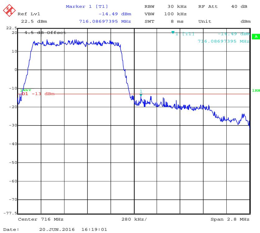
**16-QAM (1.4 MHz, FULL RB) - Left Band Edge**
