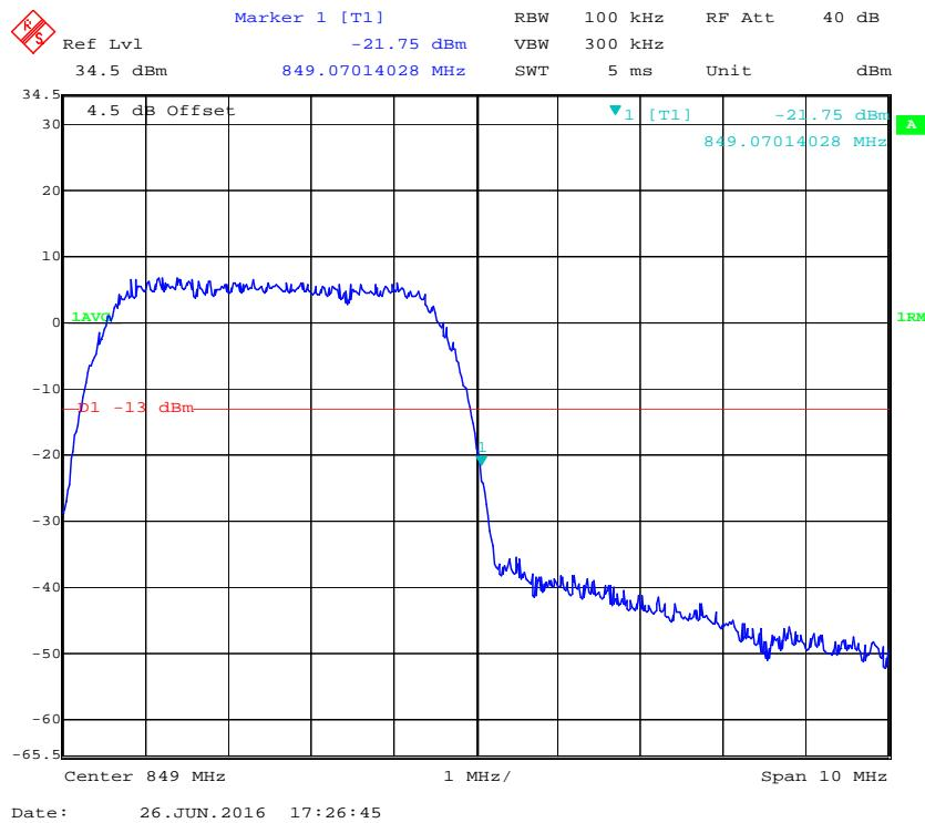
**Cellular Band, Left Band Edge for HSUPA (BPSK) Mode**
