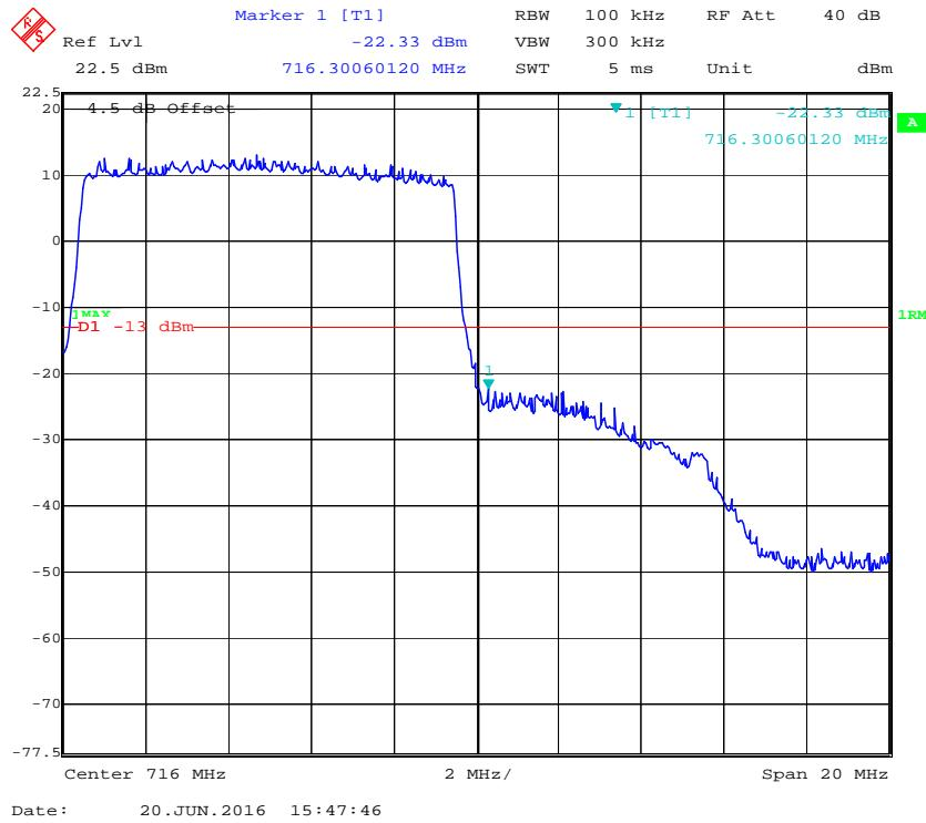
**16-QAM (10.0 MHz, FULL RB) - Left Band Edge**
