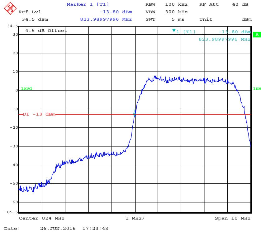
**Cellular Band, Right Band Edge for HSUPA (BPSK) Mode**
