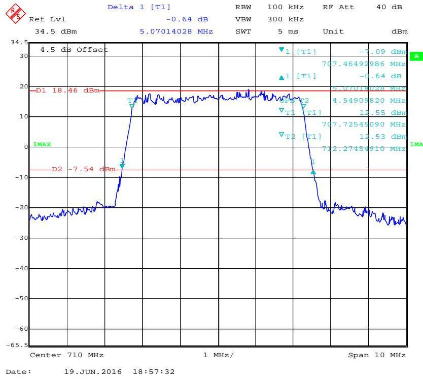
**16-QAM (5.0 MHz) - 99% Occupied Bandwidth & 26 dB Bandwidth, Middle channel**
