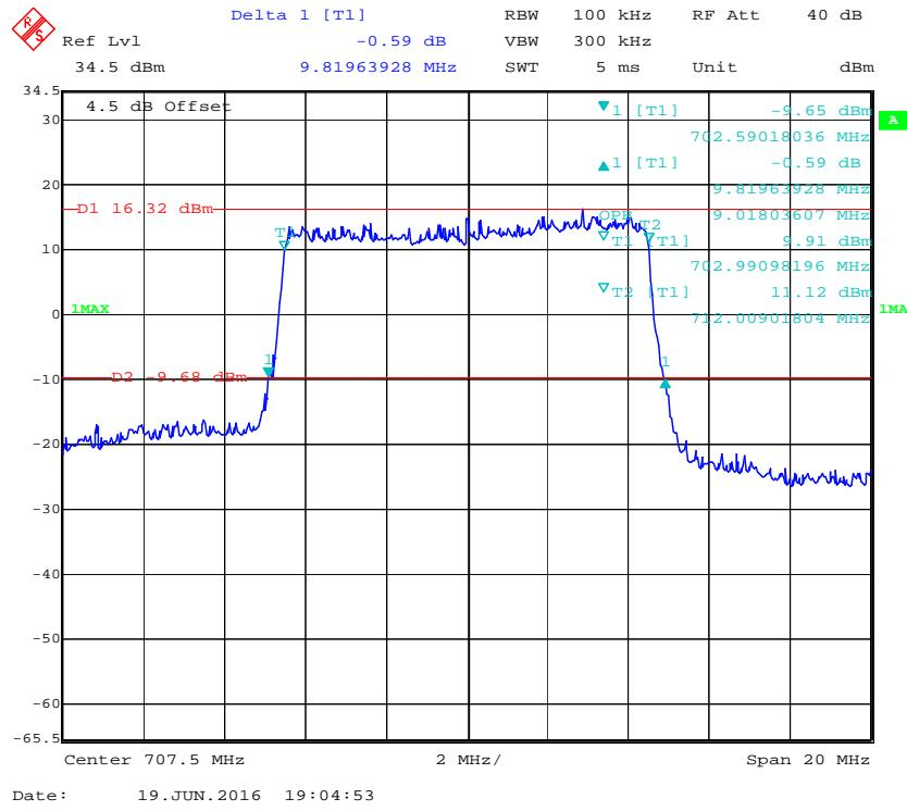
**16-QAM (10.0 MHz) - 99% Occupied Bandwidth & 26 dB Bandwidth, Middle channel**
