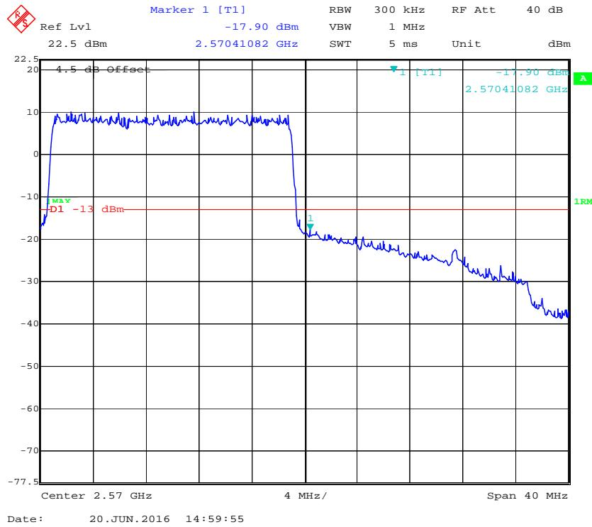
**16-QAM (20 MHz, FULL RB) - Left Band Edge**
