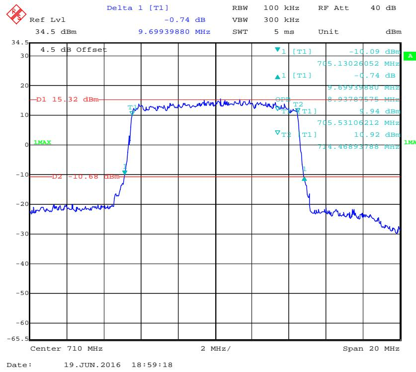
**16-QAM (10.0 MHz) - 99% Occupied Bandwidth & 26 dB Bandwidth, Middle channel**
