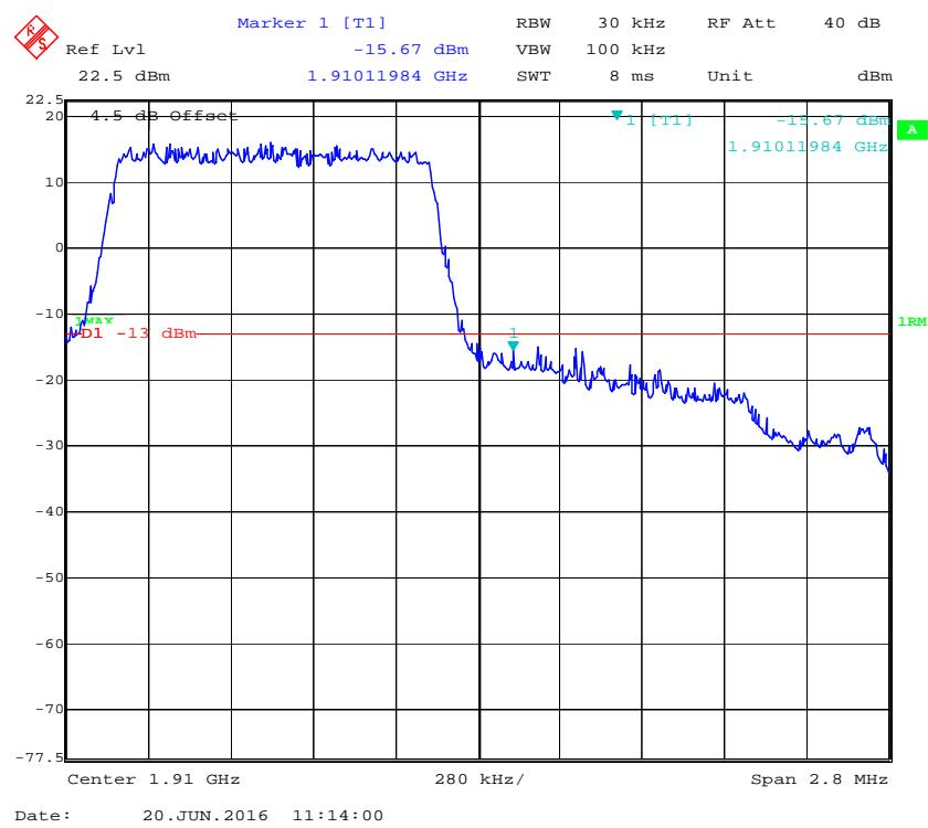
**16-QAM (1.4 MHz, FULL RB) - Left Band Edge**
