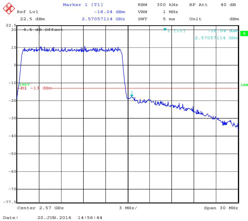
**QPSK (20 MHz, FULL RB) - Left Band Edge**
