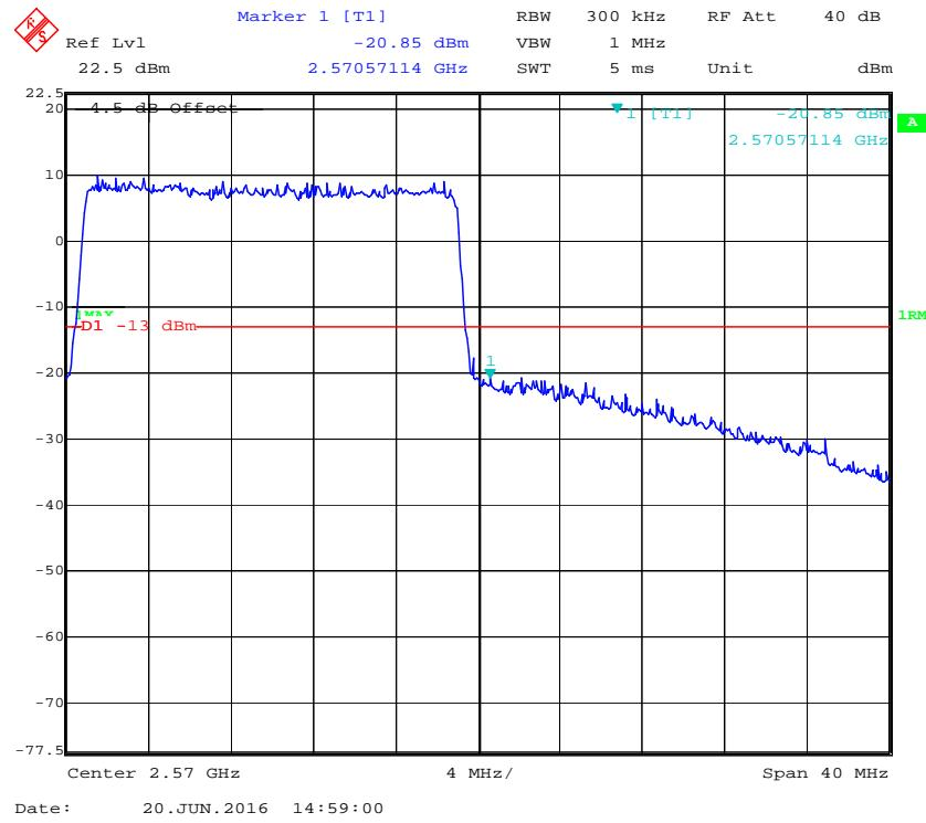
**Band 12:****QPSK (1.4 MHz, FULL RB) - Left Band Edge**
