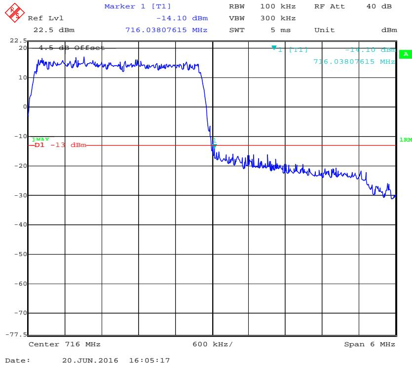
**16-QAM (5.0 MHz, FULL RB) - Left Band Edge**
