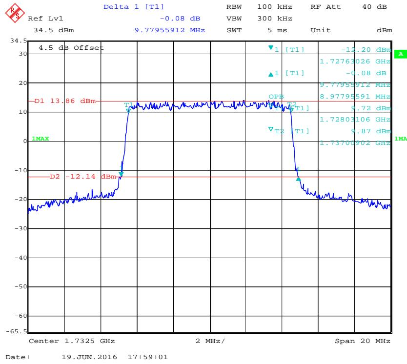
**16-QAM (10.0 MHz) - 99% Occupied Bandwidth & 26 dB Bandwidth, Middle channel**
