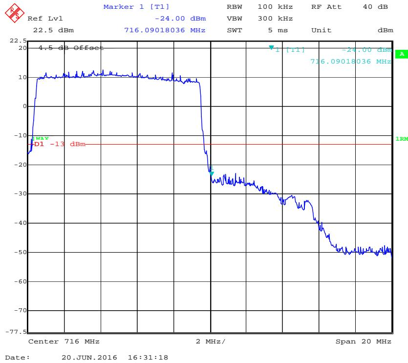
**16-QAM (10.0 MHz, FULL RB) - Left Band Edge**
