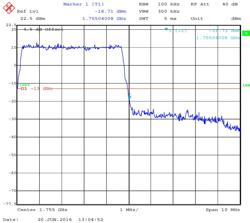
**QPSK (10.0 MHz, FULL RB) - Left Band Edge**
