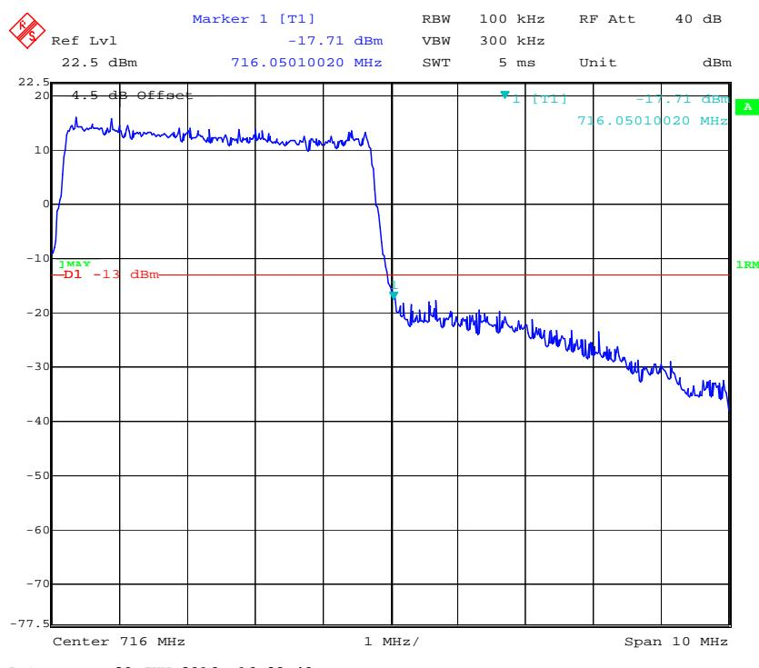
**16-QAM (5.0 MHz, FULL RB) - Left Band Edge**
