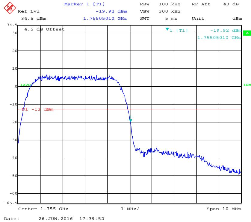
**PCS Band, Left Band Edge for HSUPA (BPSK) Mode**
