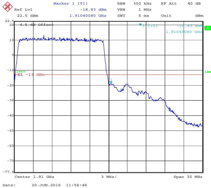
**16-QAM (15.0 MHz, FULL RB) - Left Band Edge**
