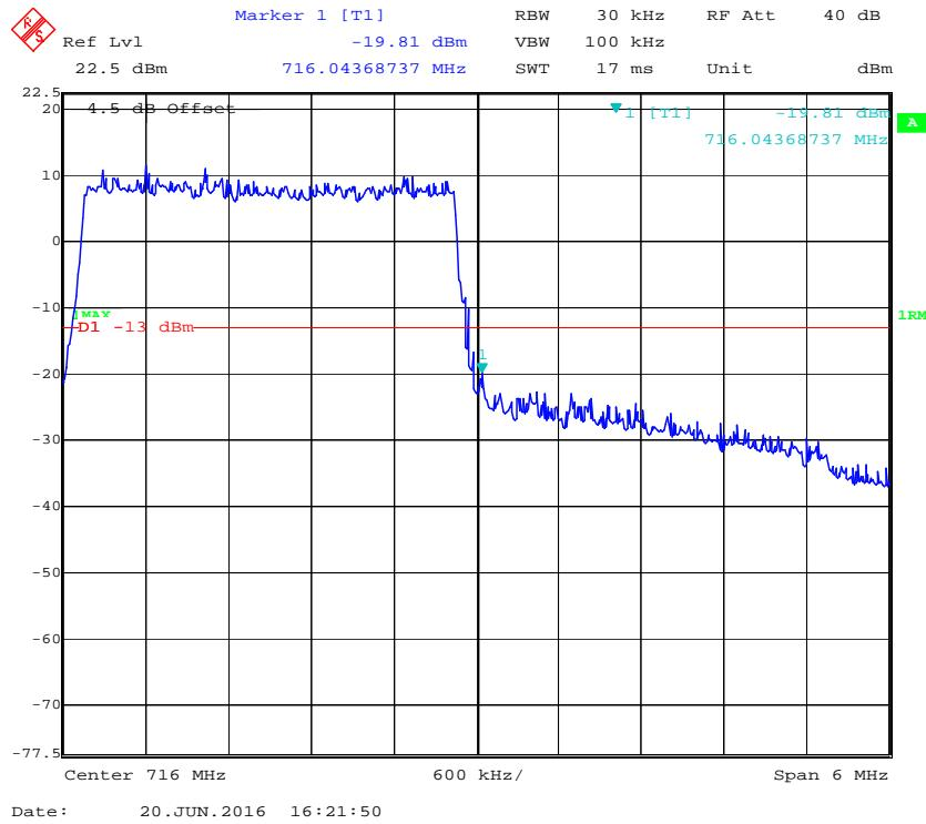
**QPSK (5.0 MHz, FULL RB) - Left Band Edge**
