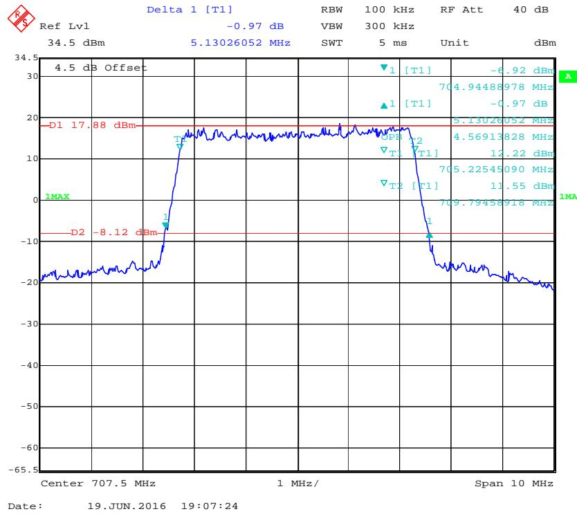
**16-QAM (5.0 MHz) - 99% Occupied Bandwidth & 26 dB Bandwidth, Middle channel**
