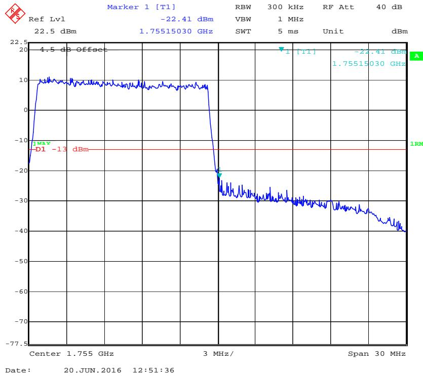
**QPSK (20.0 MHz, FULL RB) - Left Band Edge**
