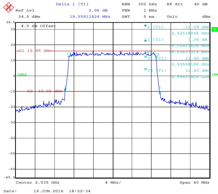
**16-QAM (20.0 MHz) - 99% Occupied Bandwidth & 26 dB Bandwidth, Middle channel**
