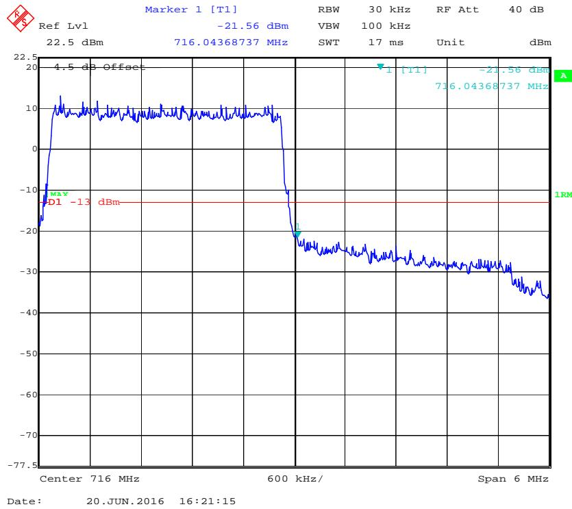
**16-QAM (3.0 MHz, FULL RB) - Left Band Edge**
