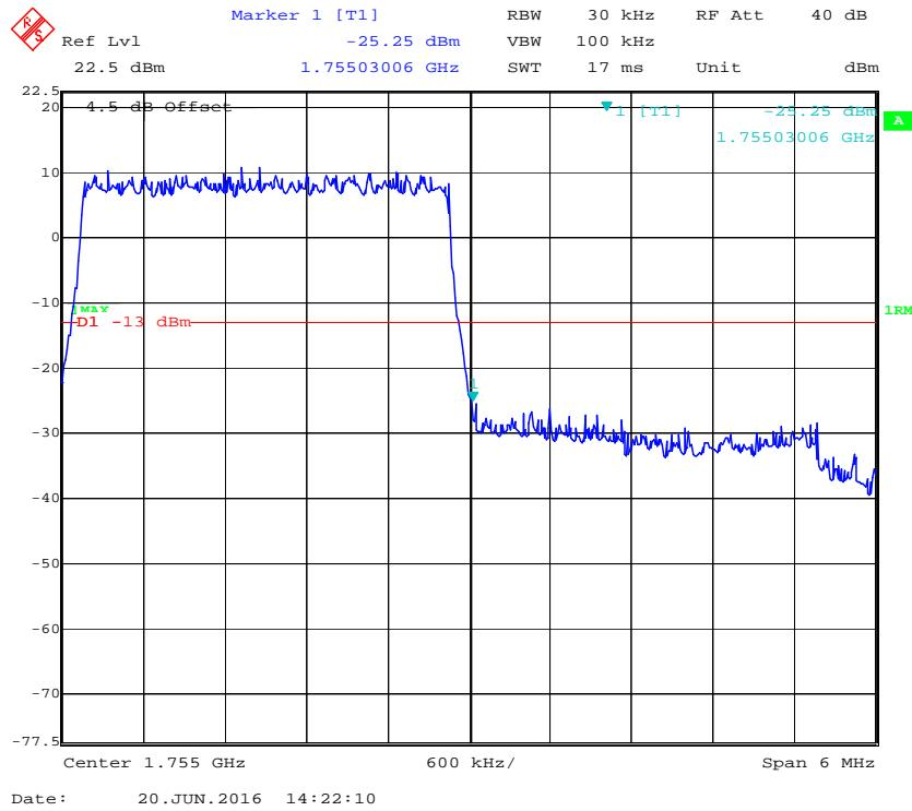
**16-QAM (3.0 MHz, FULL RB) - Left Band Edge**
