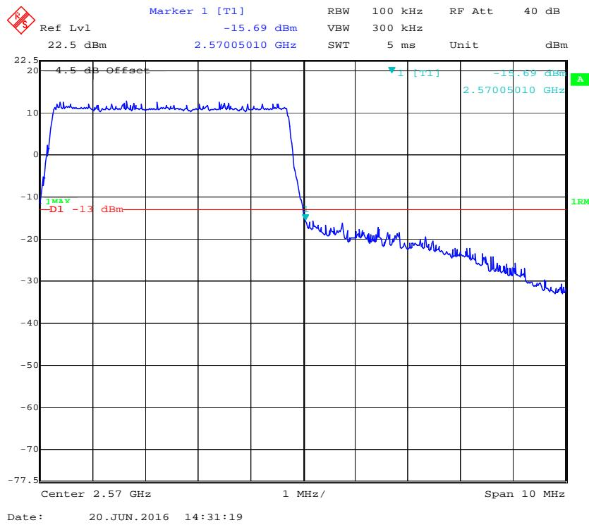
**QPSK (10.0 MHz, FULL RB) - Left Band Edge**
