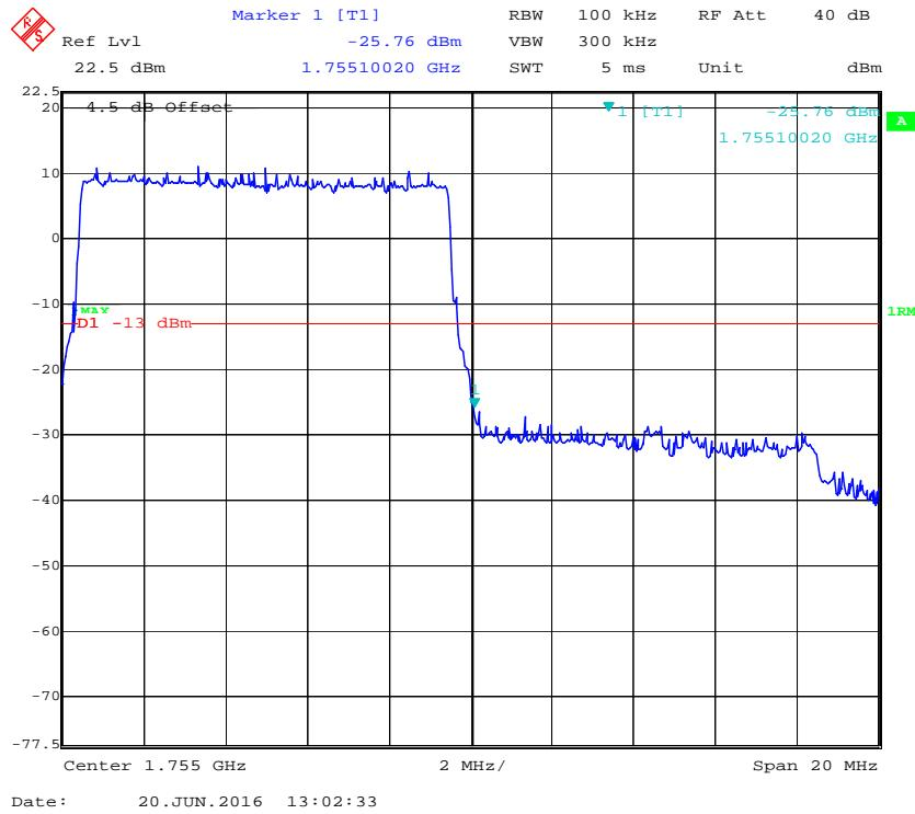
**16-QAM (10.0 MHz, FULL RB) - Left Band Edge**
