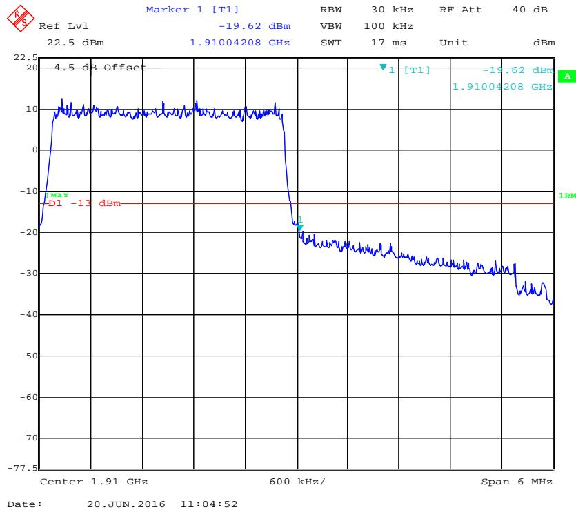
**16-QAM (3.0 MHz, FULL RB) - Left Band Edge**
