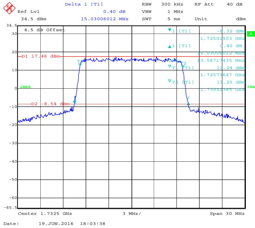
**16-QAM (15.0 MHz) - 99% Occupied Bandwidth & 26 dB Bandwidth, Middle channel**
