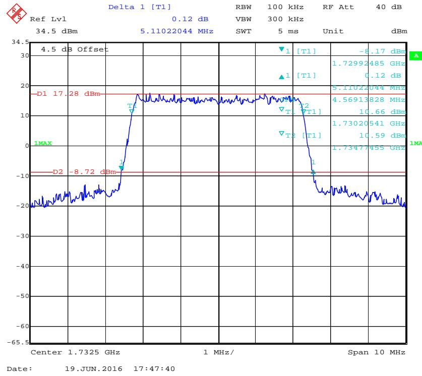
**16-QAM (5.0 MHz) - 99% Occupied Bandwidth & 26 dB Bandwidth, Middle channel**
