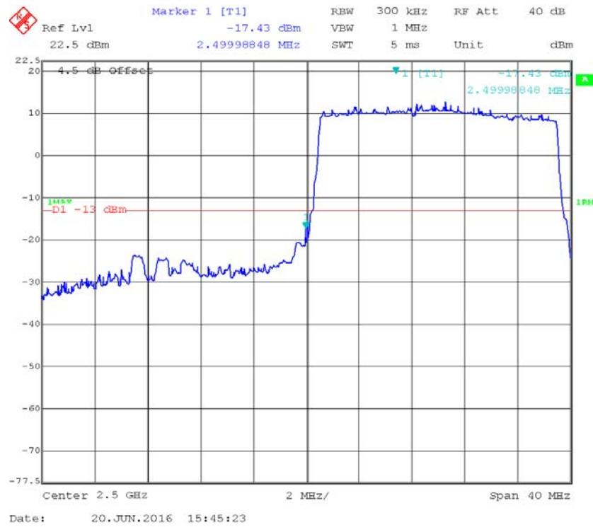
**16-QAM (20 MHz, FULL RB) - Right Band Edge**
