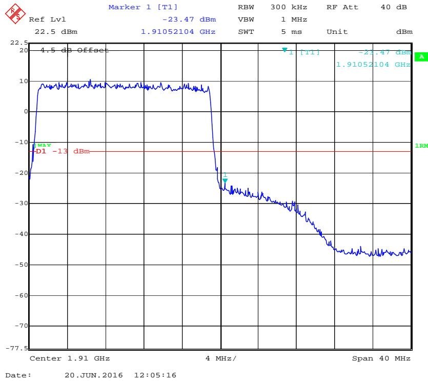
**Band 4:****QPSK (1.4 MHz, FULL RB) - Left Band Edge**
