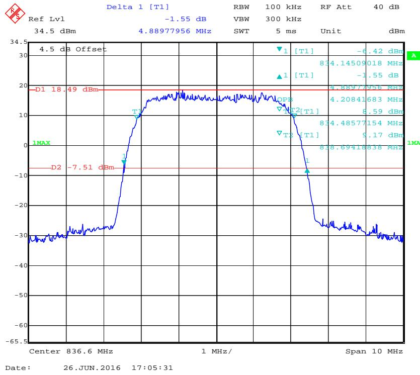
**PCS Band (Part 24E)****99% Occupied & 26 dB Emissions Bandwidth for GSM (GMSK) Mode**
