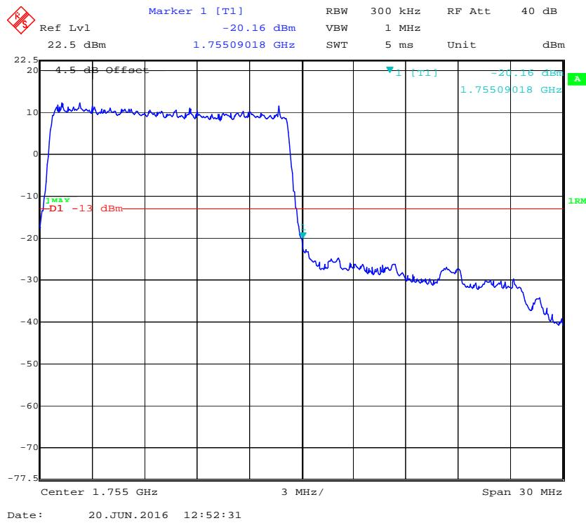
**16-QAM (15.0 MHz, FULL RB) - Left Band Edge**
