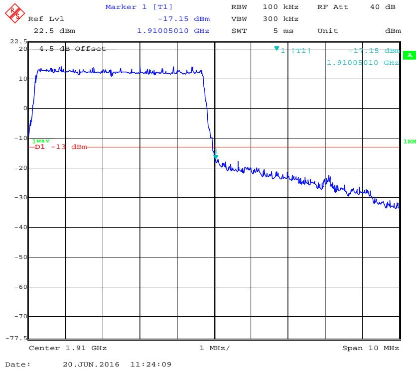
**16-QAM (5.0 MHz, FULL RB) - Left Band Edge**
