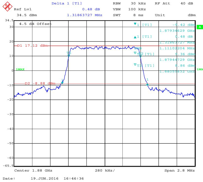
**16-QAM (1.4 MHz) - 99% Occupied Bandwidth & 26 dB Bandwidth, Middle channel**
