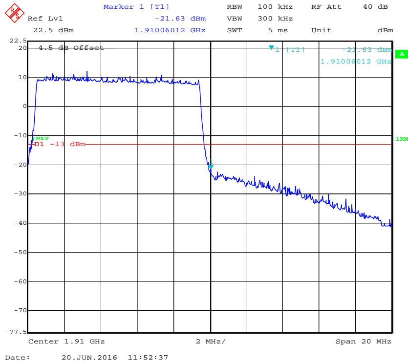
**QPSK (15.0 MHz, FULL RB) - Left Band Edge**
