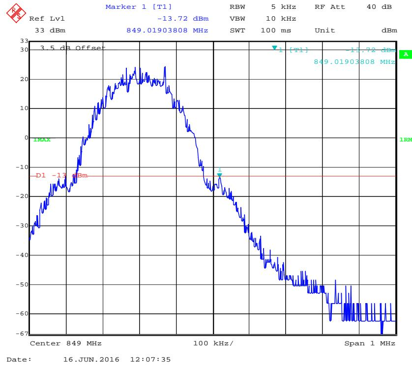
**Cellular Band, Left Band Edge for EGPRS Mode**
