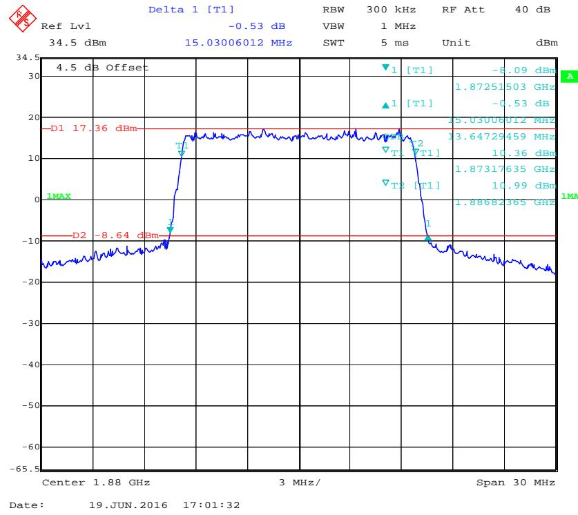
**16-QAM (15.0 MHz) - 99% Occupied Bandwidth & 26 dB Bandwidth, Middle channel**
