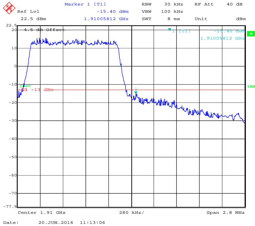
**QPSK (3.0 MHz, FULL RB) - Left Band Edge**
