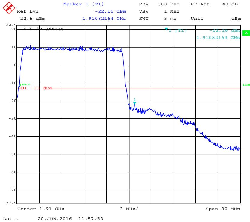
**QPSK (20.0 MHz, FULL RB) - Left Band Edge**
