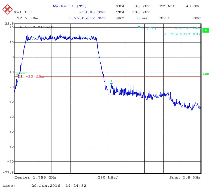
**16-QAM (1.4 MHz, FULL RB) - Left Band Edge**
