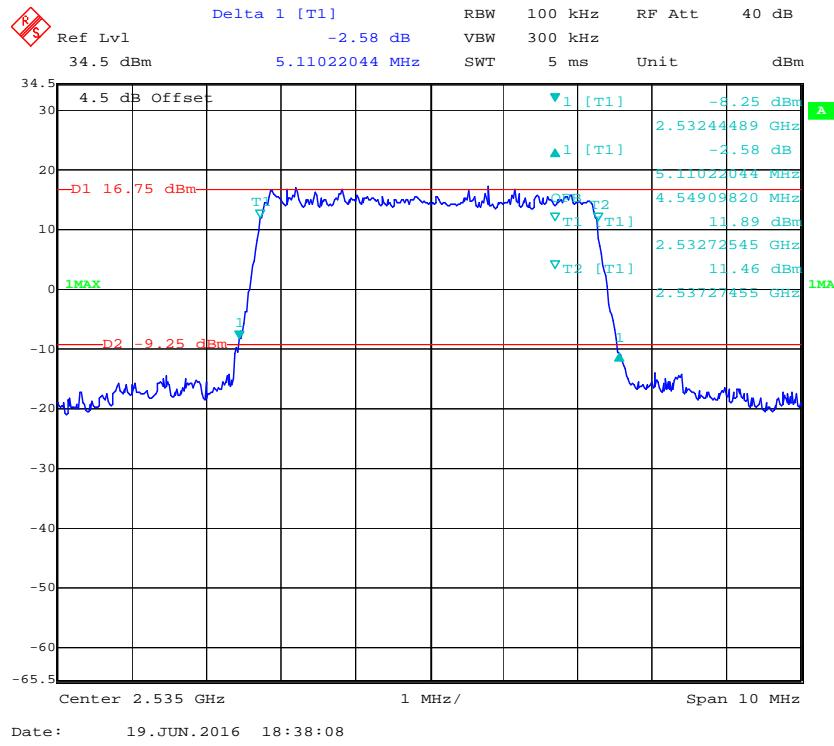
**16-QAM (5.0 MHz) - 99% Occupied Bandwidth & 26 dB Bandwidth, Middle channel**
