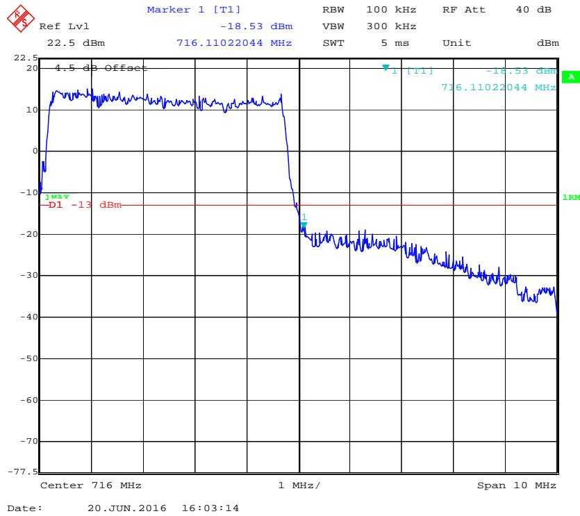
**QPSK (10.0 MHz, FULL RB) - Left Band Edge**
