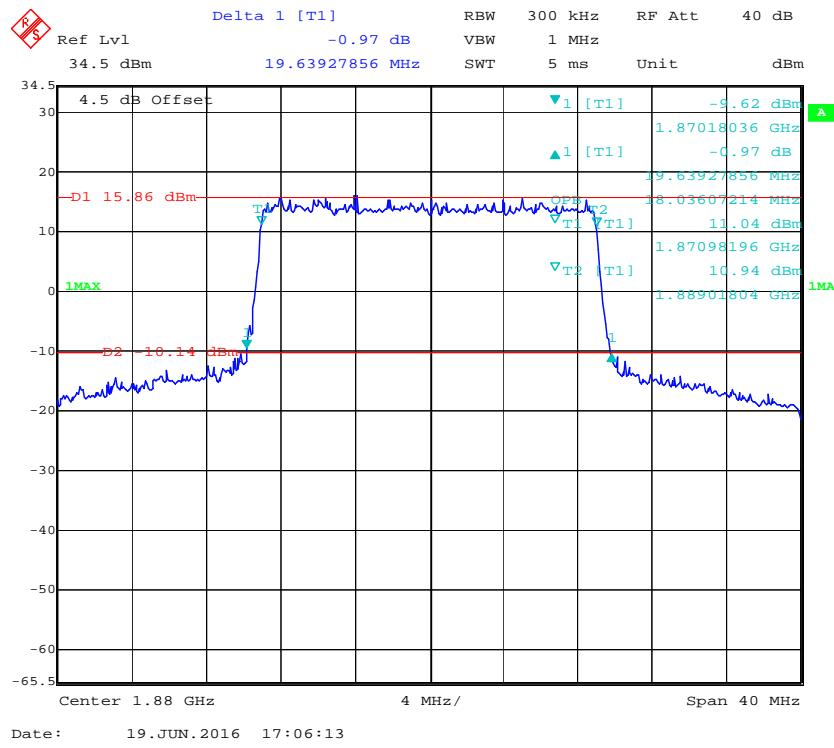
**16-QAM (20.0 MHz) - 99% Occupied Bandwidth & 26 dB Bandwidth, Middle channel**
