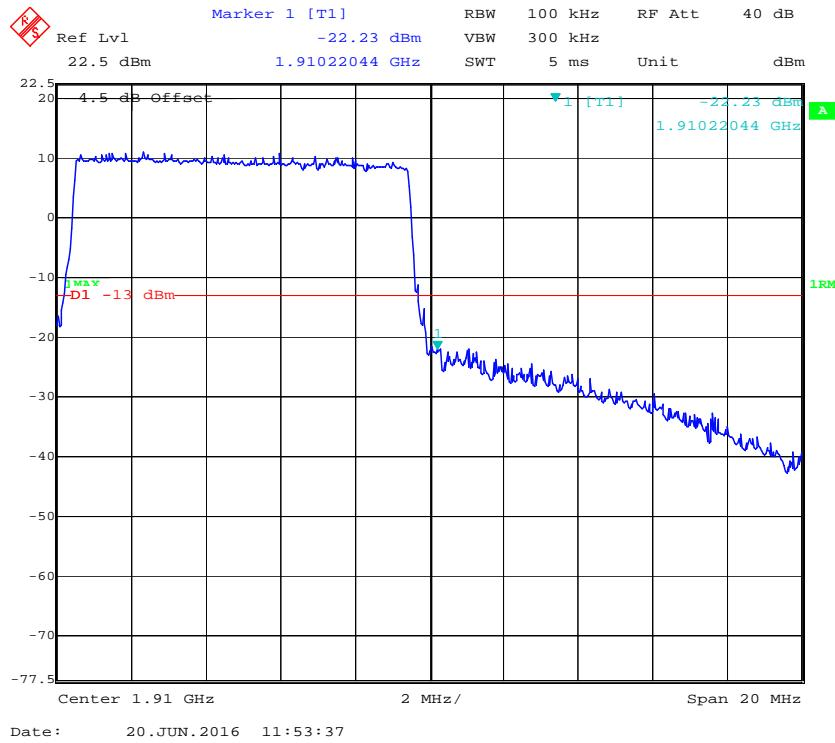
**16-QAM (10.0 MHz, FULL RB) - Left Band Edge**
