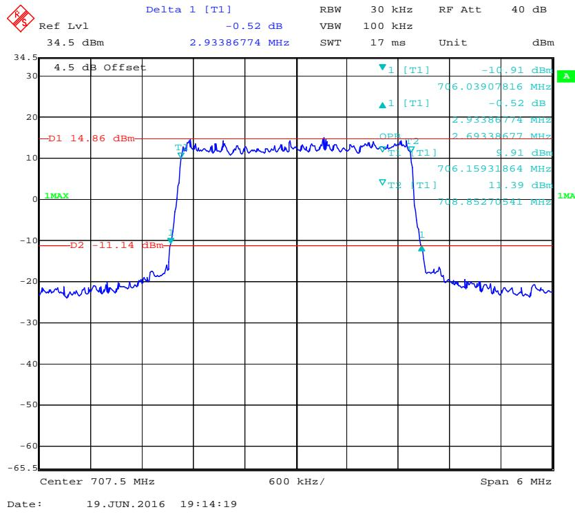
**16-QAM (3.0MHz) - 99% Occupied Bandwidth & 26 dB Bandwidth, Middle channel**
