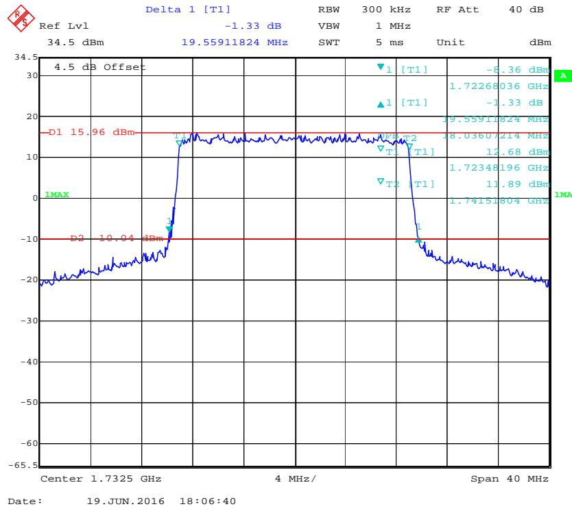
**16-QAM (20.0 MHz) - 99% Occupied Bandwidth & 26 dB Bandwidth, Middle channel**
