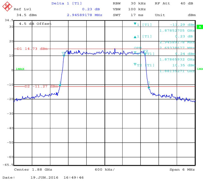
**16-QAM (3.0 MHz) - 99% Occupied Bandwidth & 26 dB Bandwidth, Middle channel**
