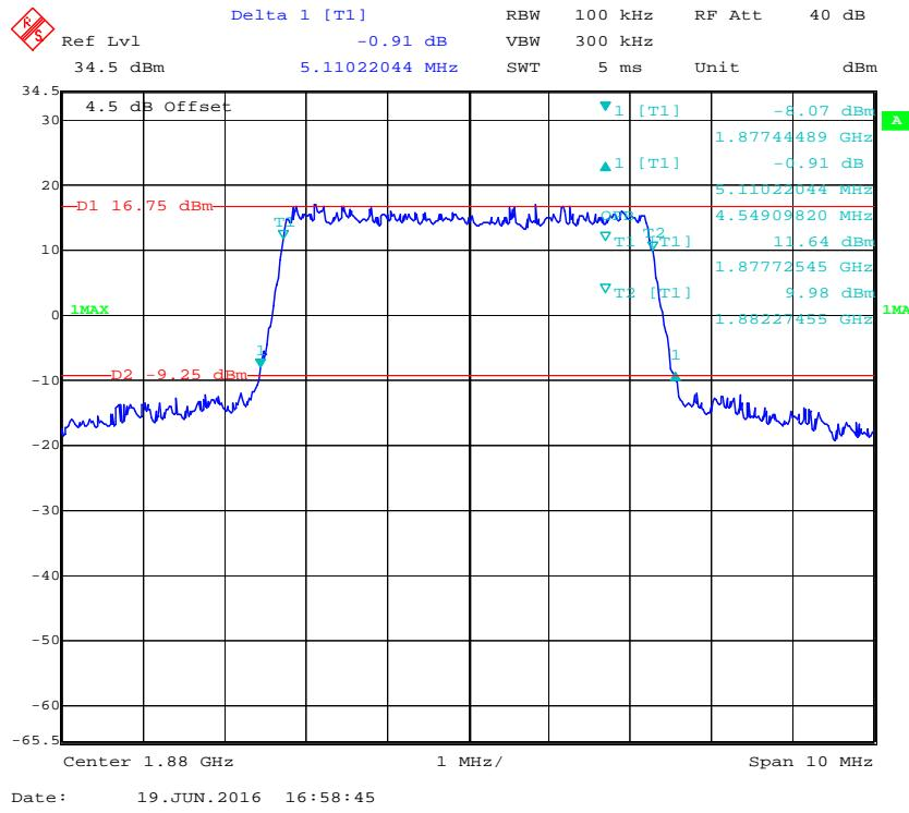
**16-QAM (5.0 MHz) - 99% Occupied Bandwidth & 26 dB Bandwidth, Middle channel**
