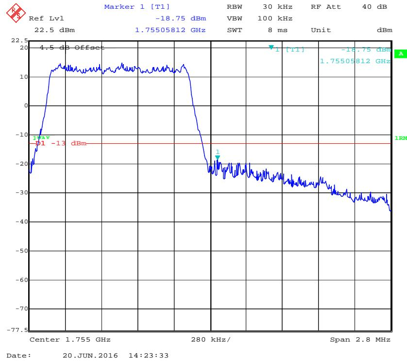
**QPSK (3.0 MHz, FULL RB) - Left Band Edge**
