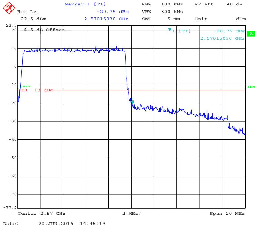
**16-QAM (10.0 MHz, FULL RB) - Left Band Edge**
