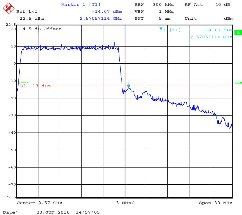
**16-QAM (15 MHz, FULL RB) - Left Band Edge**
