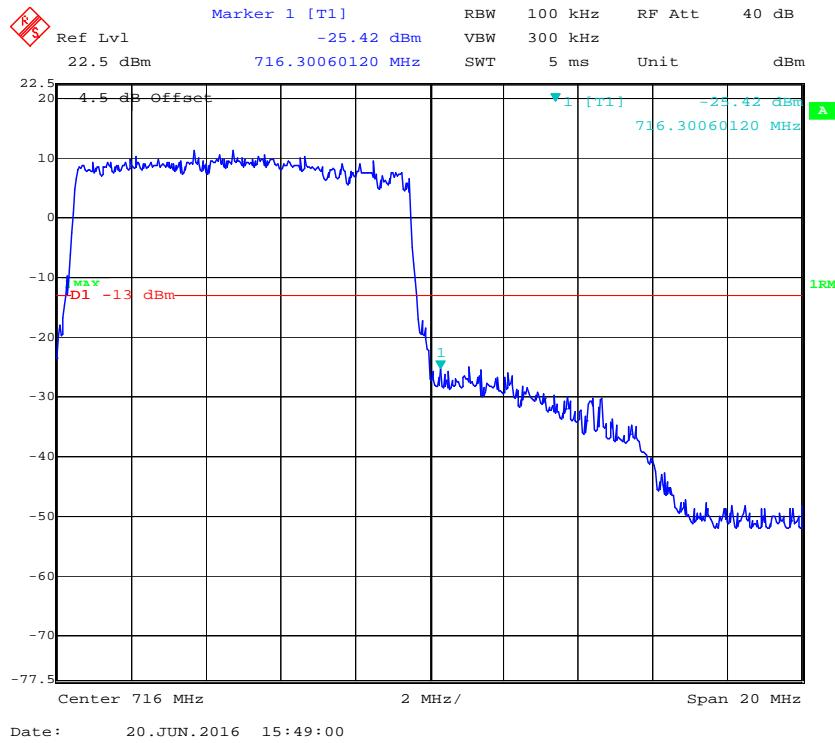
**Band 17:****QPSK (5.0 MHz, FULL RB) - Left Band Edge**
