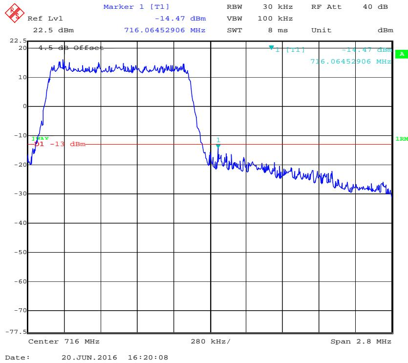
**QPSK (3.0 MHz, FULL RB) - Left Band Edge**
