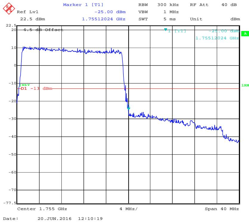
**16-QAM (20.0 MHz, FULL RB) - Left Band Edge**
