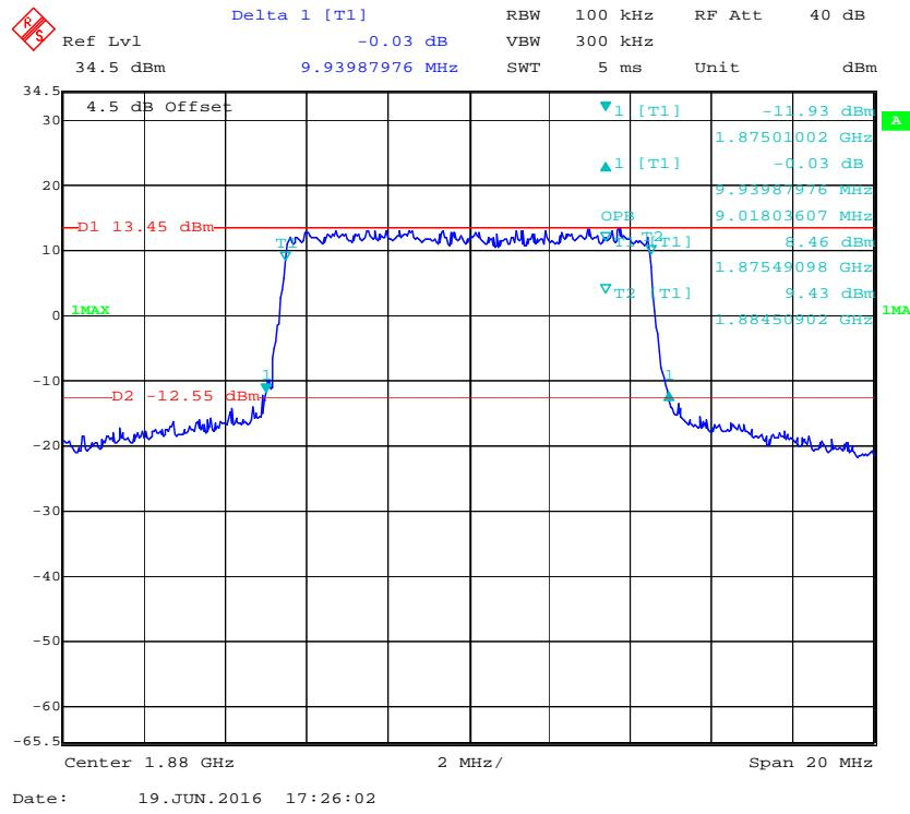
**16-QAM (10.0 MHz) - 99% Occupied Bandwidth & 26 dB Bandwidth, Middle channel**
