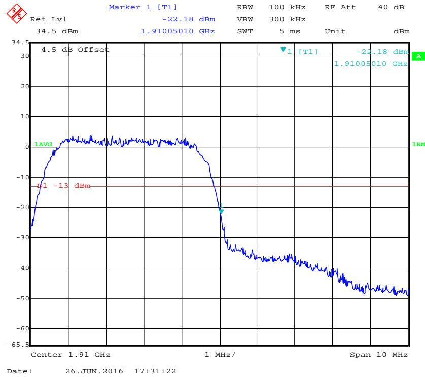
**PCS Band, Left Band Edge for HSUPA (BPSK) Mode**
