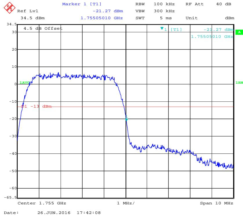
**Band 2:****QPSK (1.4 MHz, FULL RB) - Left Band Edge**
