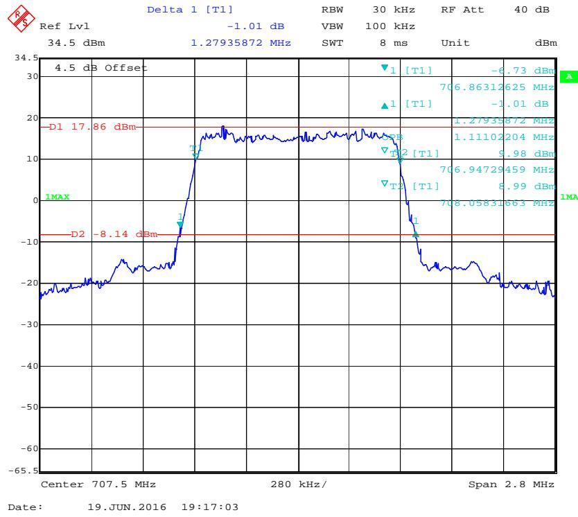
**16-QAM (1.4 MHz) - 99% Occupied Bandwidth & 26 dB Bandwidth, Middle channel**
