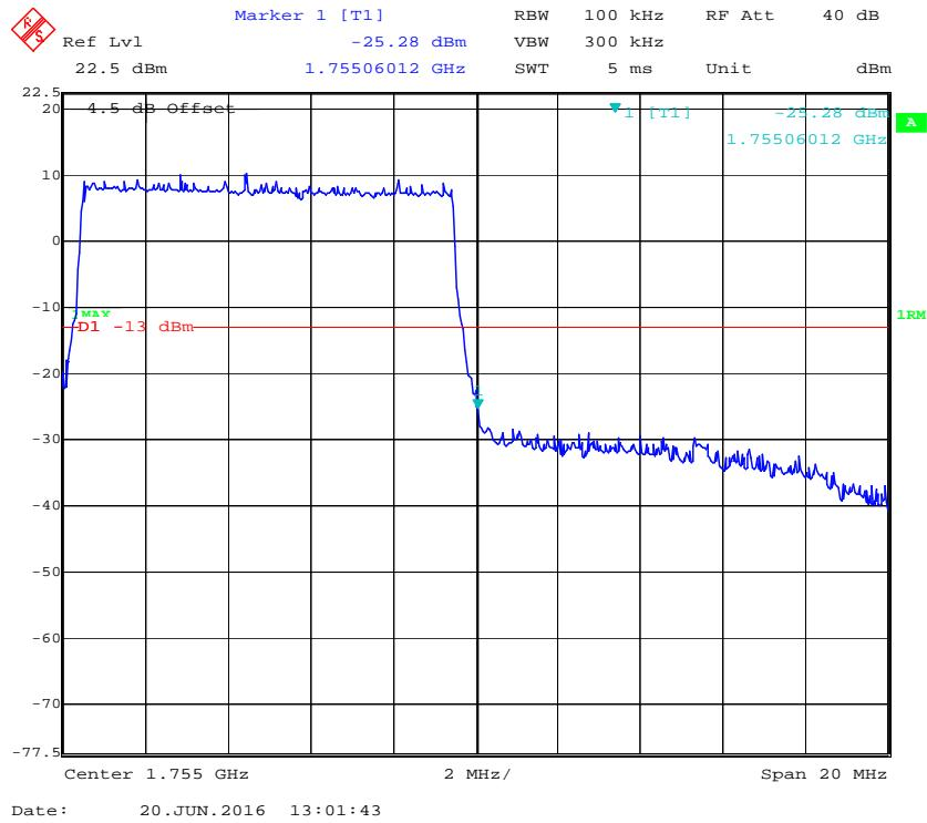
**QPSK (15.0 MHz, FULL RB) - Left Band Edge**
