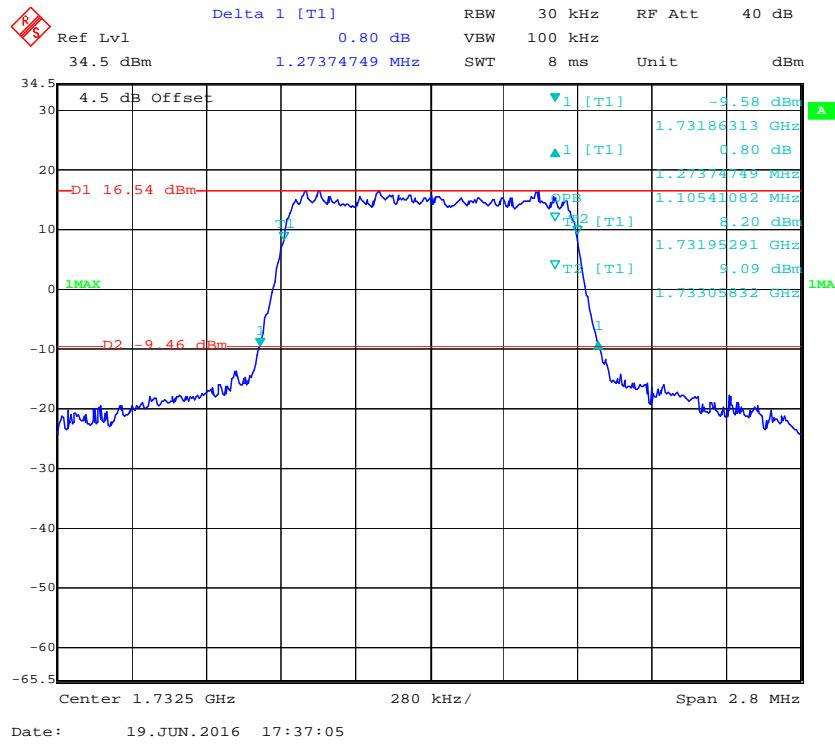
**16-QAM (1.4 MHz) - 99% Occupied Bandwidth & 26 dB Bandwidth, Middle channel**
