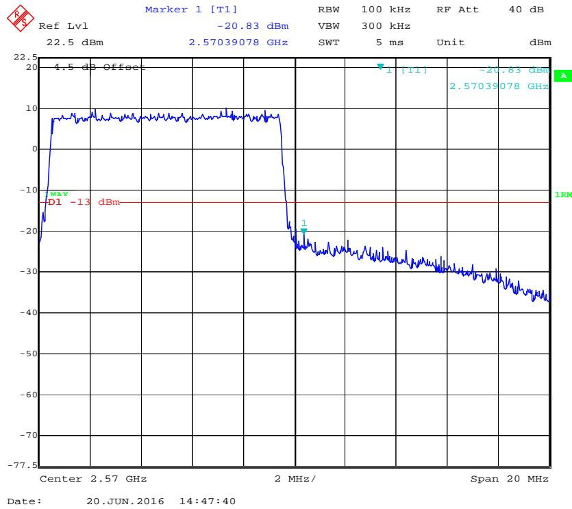
**QPSK (15 MHz, FULL RB) - Left Band Edge**
