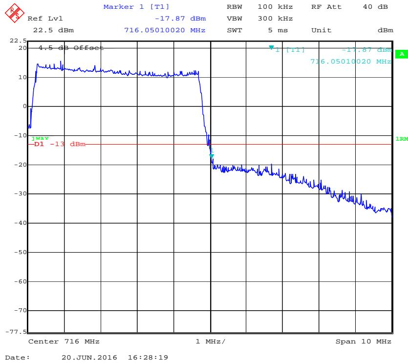
**QPSK (10.0 MHz, FULL RB) - Left Band Edge**
