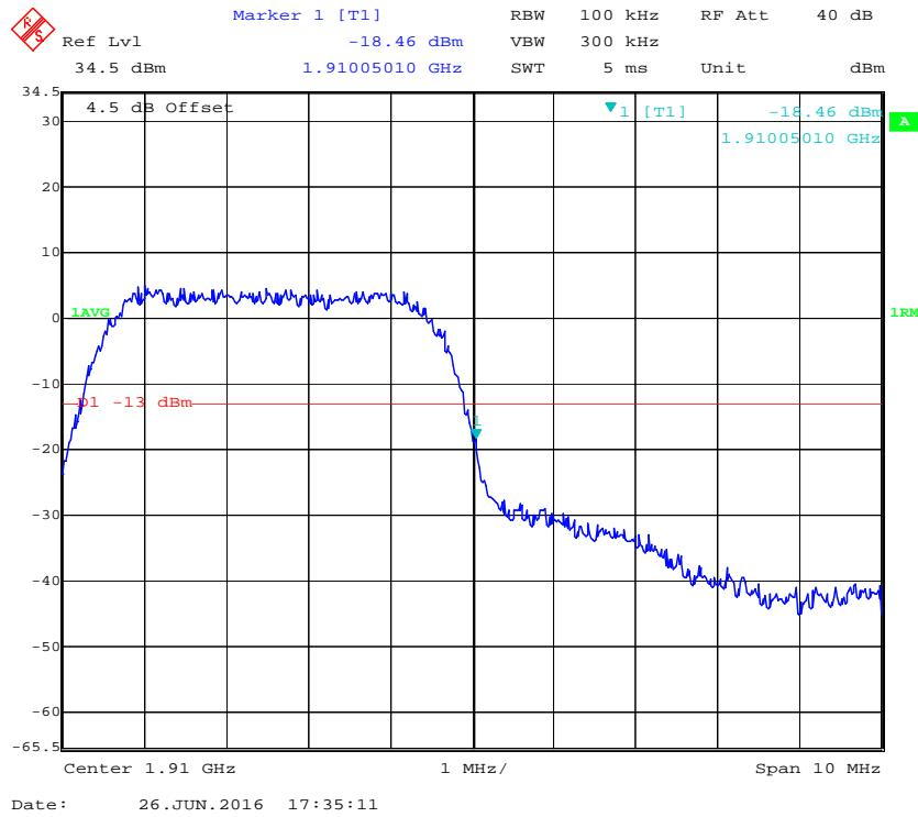
**PCS Band, Left Band Edge for HSDPA (16QAM) Mode**
