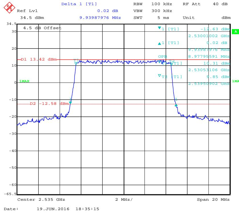
**16-QAM (10.0MHz) - 99% Occupied Bandwidth & 26 dB Bandwidth, Middle channel**
