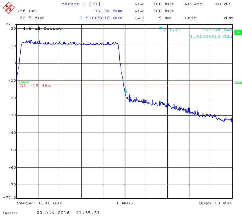
**QPSK (10.0 MHz, FULL RB) - Left Band Edge**
