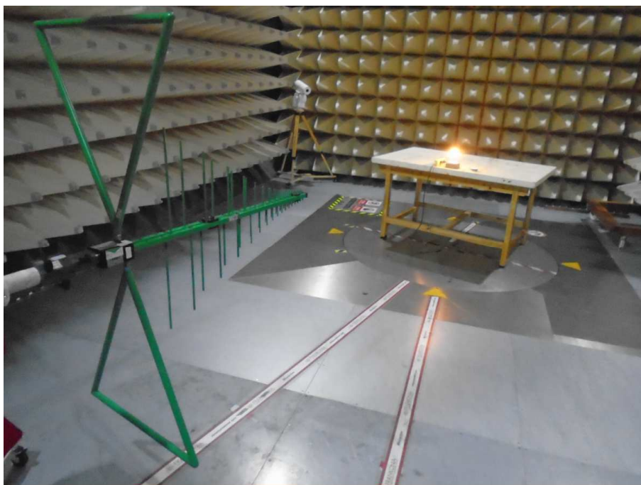
Photograph 2: Set-up for measurement of radiated emission
