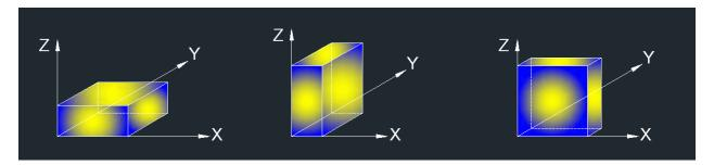
Note 1: For below 1GHz radiated test, EUT in each of three orthogonal axis emissions had been tested, but only the worst case (X axis) data recorded in the report.
