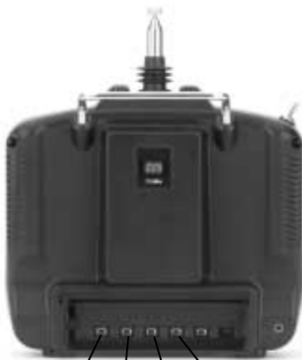
Throttle Aileron Elevator Rudder Servo Reversing Switches (Located behind Transmitter Battery Pack)
