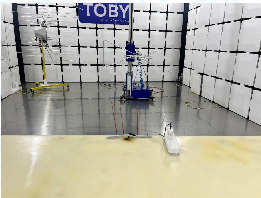
Photo of Setup for Radiated Emission (30MHz~1GHz)
