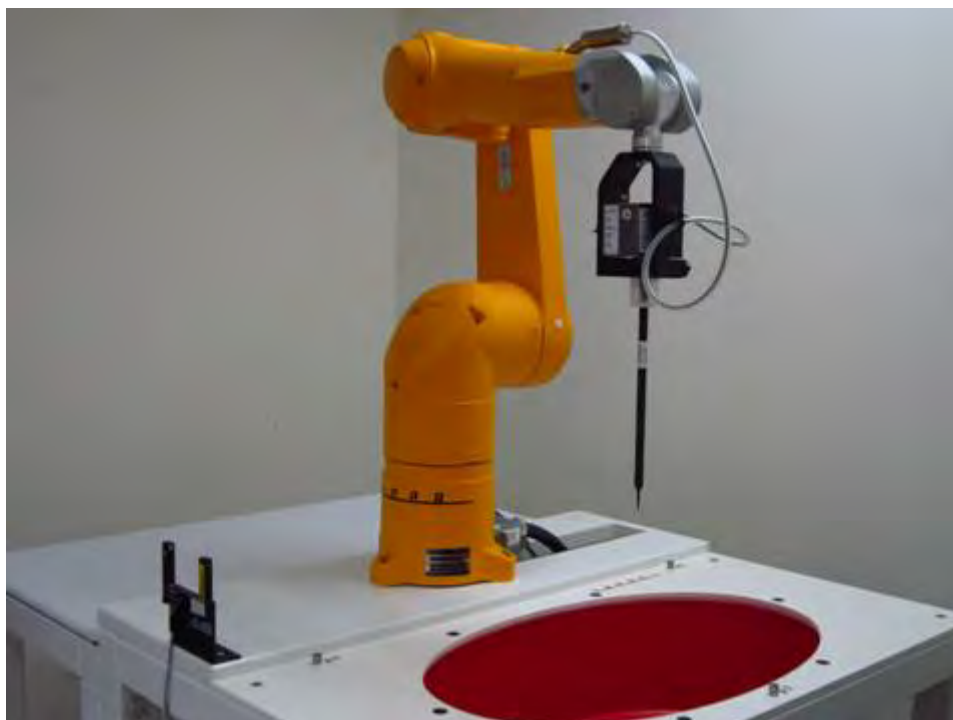
Fig.1 Photograph of the SAR measurement system
