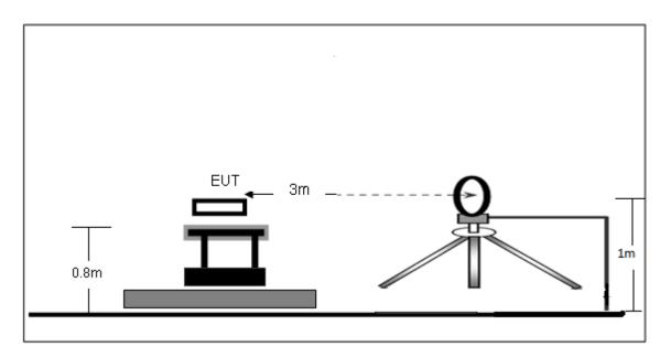
(B) Radiated Emission Test-Up Frequency 30MHz~1GHz
