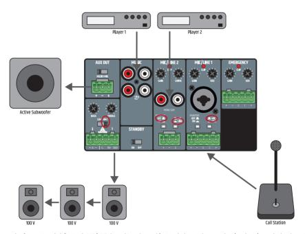
The connection for a mute switch/button in MIC/LINE channel 1 can be used for two devices at the same time (muting of a music signal or activation of the gong/signal tone). In this case, the mute contacts of both devices must be connected to poles C and + of the terminal strip connections for MIC/LINE 1.
