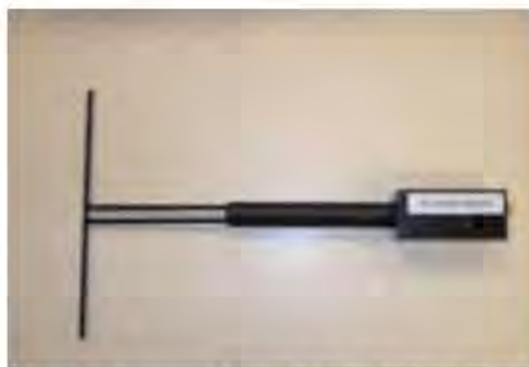
Figure 1 – Satimo COMOSAR Validation Dipole
