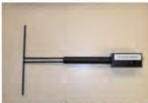
Figure 1 – Satimo COMOSAR Validation Dipole
