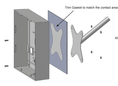
Attach the box with the gasket to the mount
