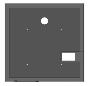
Modify the gasket to the match the large holes on the mounting plate and to match the area between the mount and the box, to create a seal against the elements (see below).
